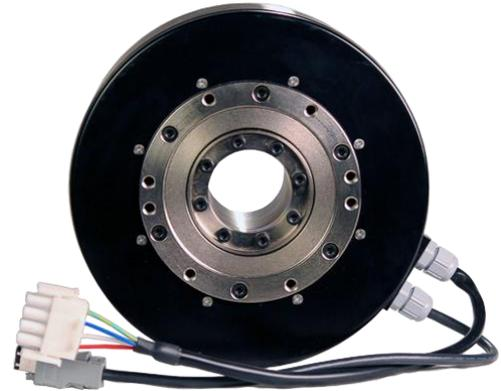
The chief advantage of direct drive products is the ability to attach a load directly to the servo motor, allowing a full range of motion control without the need for a shaft coupling or gearhead. SGM7F also offers a superior level of torsional stiffness and virtually eliminates mechanical backlash. This yields an output that minimizes damage to components and maximizes positioning accuracy and repeatability. The SGM7F also offers a host of other advantages, including:
