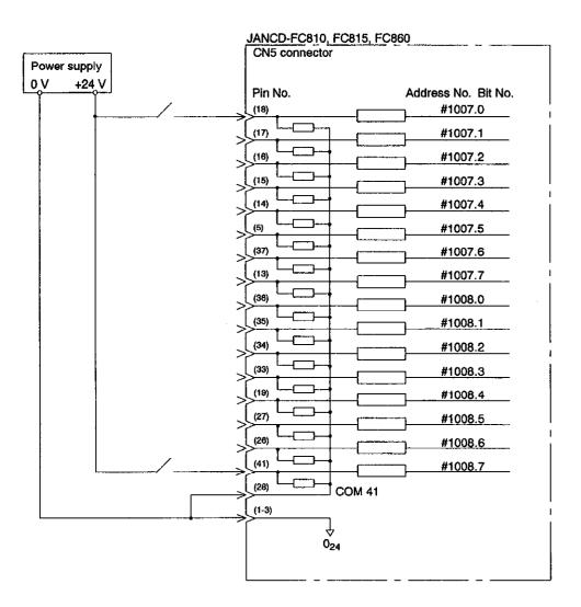
Fig. 11.7 FC810, FC815, FC860 Module Connection (Address number and bit number: #1007.0 to #1008.7)
