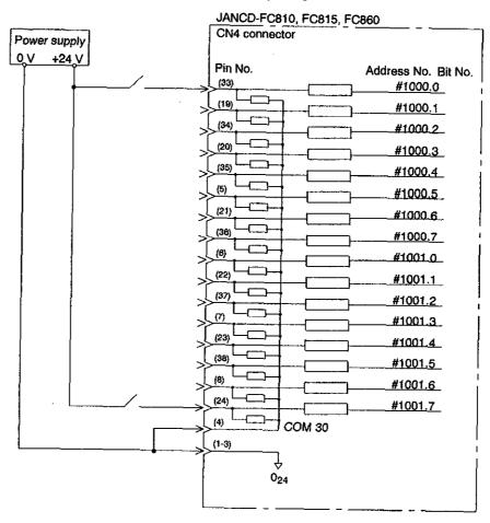
Fig. 11.3 FC810, FC815, FC860 Module Connection (Address number and bit number: #1000.0 to #1001.7)
