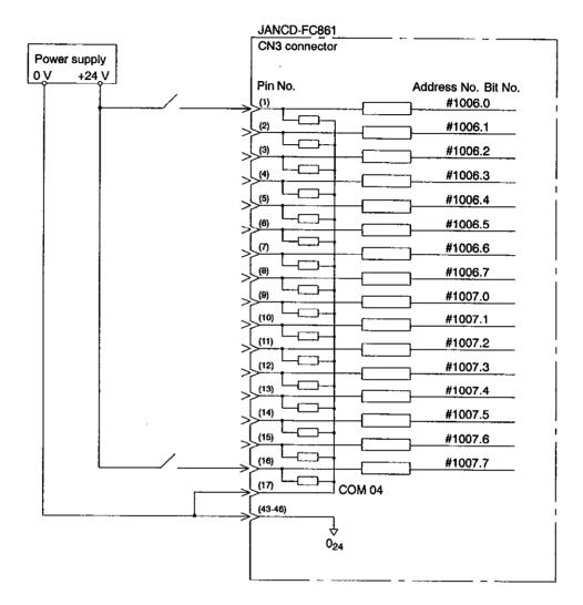
Fig. 11.30 FC861 Module Connection (Address number and bit number: #1006.0 to #1007.7)
