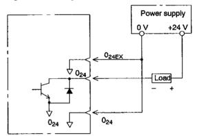
Fig. 11.50 Output Circuit (When using external power)
