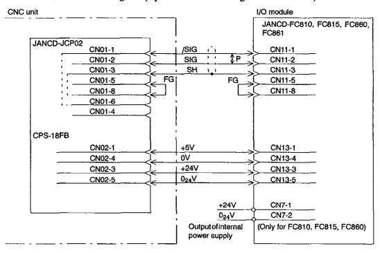
Fig. 10.2 Detailed Connection of I/O Module
