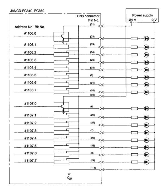
Fig. 11.16 FC810/FC860 Module Connection (Address number and bit number: #1106.0 to #1107.7)
