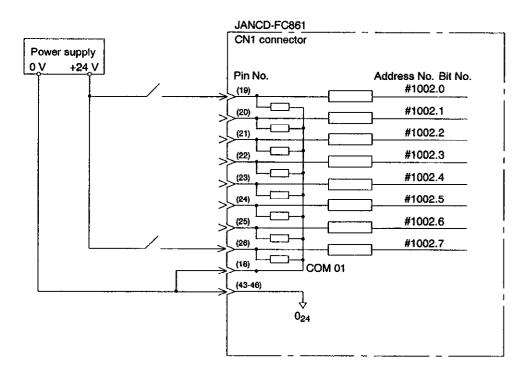
Fig. 11.27 FC861 Module Connection (Address number and bit number: #1002.0 to #1002.7)
