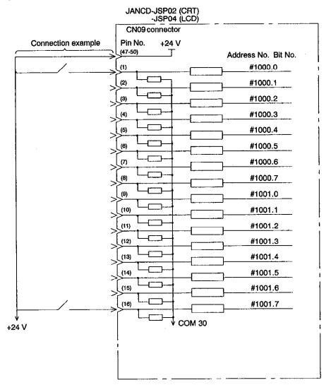
The I/O port in JSP02 module and the one in JSP04 module are compatible with each other.
