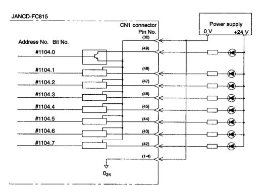
Fig. 11.21 FC815 Module Connection (Address number and bit number: #1104.0 to #1104.7)
