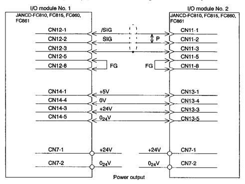
Fig. 10.4 Detailed Connection of Additional I/O Module
