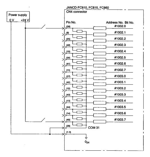
Fig. 11.4 FC810, FC815, FC860 Module Connection (Address number and bit number: #1002.0 to #1003.7)
