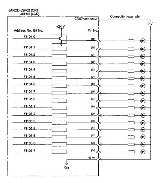
Fig. 11.42 JSP02/JSP04 Module Connection (Address number and bit number: #1104.0 to #1105.7)
