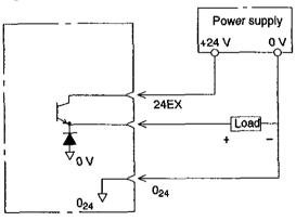
Fig. 11.48 Output Circuit (When using external power)
