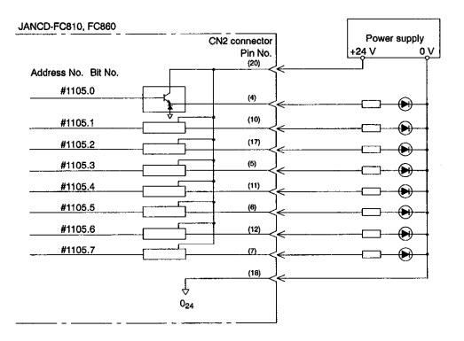
Fig. 11.15 FC810/FC860 Module Connection (Address number and bit number: #1105.0 to #1105.7)
