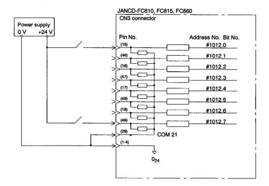
Fig. 11.10 FC810, FC815, FC860 Module Connection (Address number and bit number: #1012.0 to #1012.7)
