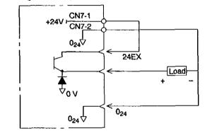
Fig. 11.47 Output Circuit (When using internal power)
