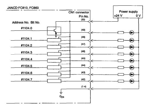
Fig. 11.14 FC810/FC860 Module Connection (Address number and bit number: #1104.0 to #1104.7)
