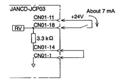
Fig. 9.6 Input Circuit
