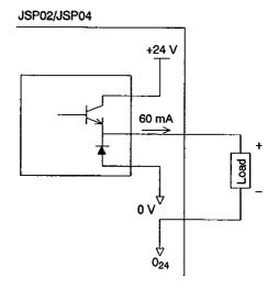
Fig. 11.56 Output Circuit
