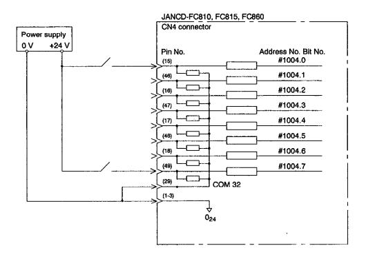
Fig. 11.5 FC810, FC815, FC860 Module Connection (Address number and bit number: #1004.0 to #1004.7)
