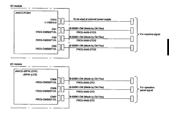
Fig. 11.2 Connection between Devices
