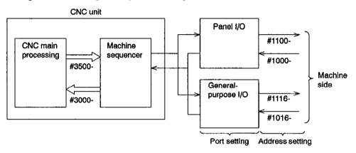
Fig. 11.44 CNC Unit and External Signals
