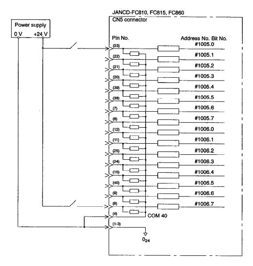
Fig. 11.6 FC810, FC815, FC860 Module Connection (Address number and bit number: #1005.0 to #1006.7)
