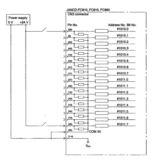
Fig. 11.9 FC810, FC815, FC860 Module Connection (Address number and bit number: #1010.0 to #1011.7)
