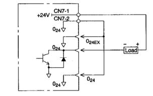
Fig. 11.49 Output Circuit (When using internal power)
