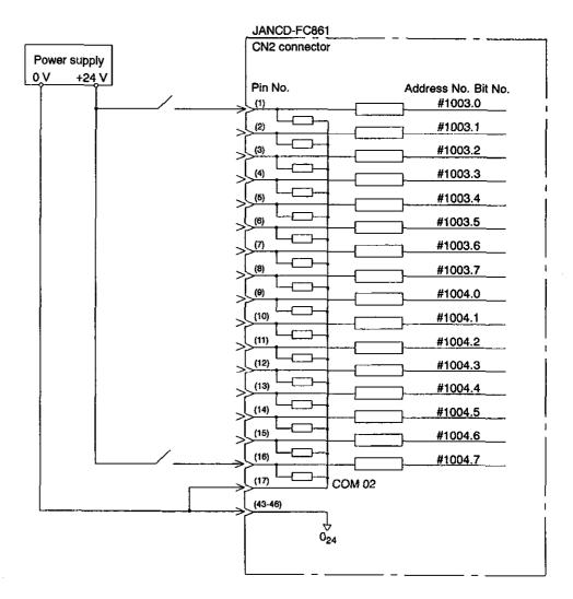
Fig. 11.28 FC861 Module Connection (Address number and bit number: #1003.0 to #1004.7)
