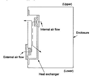
Fig. 1.7 Mounting of Heat Exchanger
