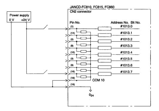
Fig. 11.11 FC810, FC815, FC860 Module Connection (Address number and bit number: #1013.0 to #1013.7)
