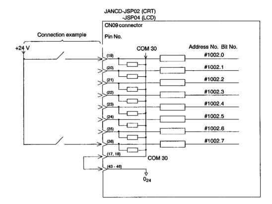
Fig. 11.36 JSP02/JSP04 Module Connection (Address number and bit number: #1002.0 to #1002.7)
