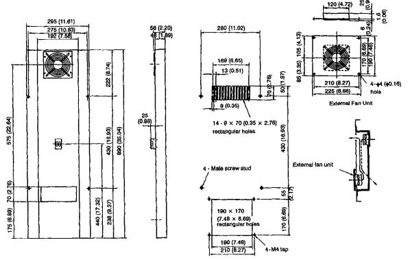
Mounting Hole Machining Drawing
