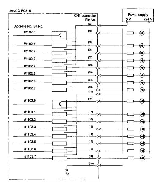
Fig. 11.20 FC815 Module Connection (Address number and bit number: #1102.0 to #1103.7)
