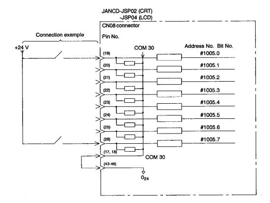
Fig. 11.38 JSP02/JSP04 Module Connection (Address number and bit number: #1005.0 to #1005.7)
