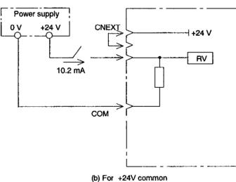
Fig. 11.52 Input Circuit (When using external power)
