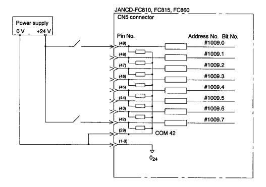
Fig. 11.8 FC810, FC815, FC860 Module Connection (Address number and bit number: #1009.0 to #1009.7)
