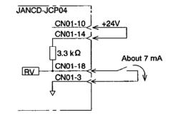
Fig. 9.5 Input Circuit
