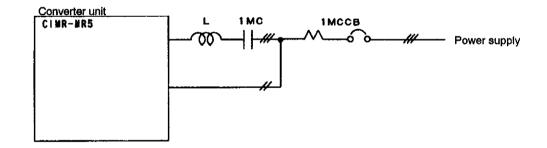
Fig. 3.2 Connection between Devices
