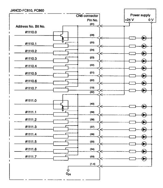
Fig. 11.18 FC810/FC860 Module Connection (Address number and bit number: #1110.0 to #1111.7)
