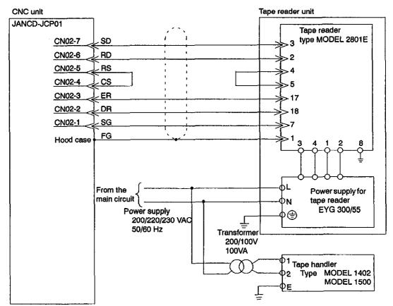
When the tape reader of MODEL 2801E is used, connect it in the manner shown in Fig. 8.3.
