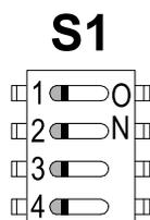
Figure 5.1 Default Settings for DIP Switch S1
