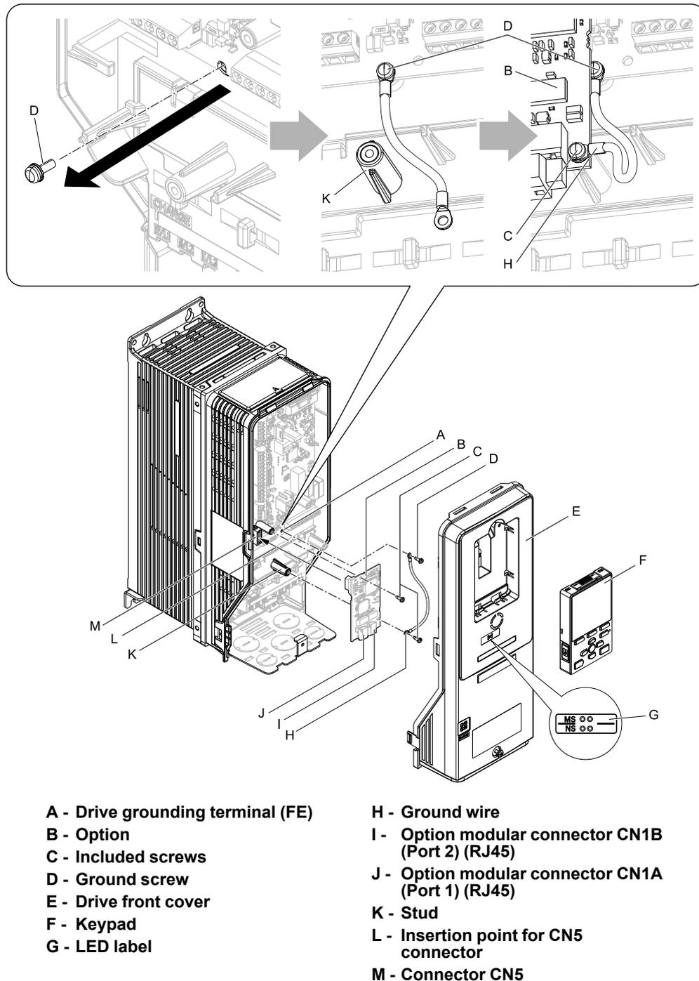
Figure 5.7 Drive Components with Option
