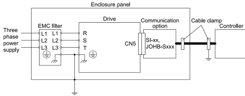
Figure 11.3 Option Installation for CE Compliance: GA500, HV600
