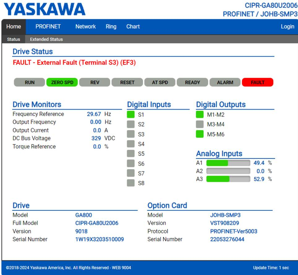
**Figure 9.2 Home Page View (Fault/Minor Fault)**
