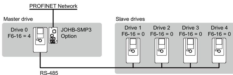
Figure 8.3 Gateway Mode Setup
