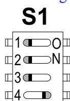
Figure 5.2 PROFINET Settings for DIP Switch S1
