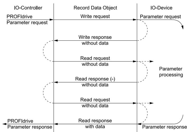
**Figure 8.4 PROFIdrive Acyclic Parameter Access Mechanism Structure**
