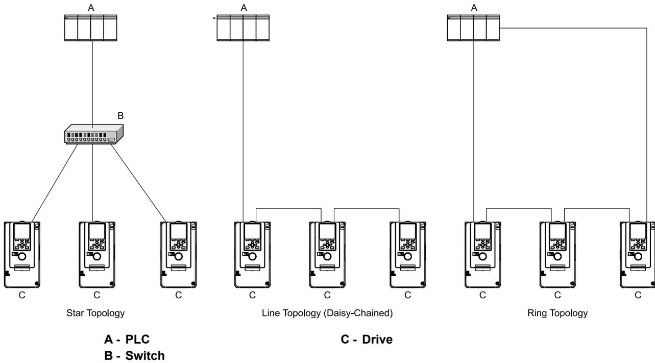
Figure 5.9 Communication Cable Wiring
