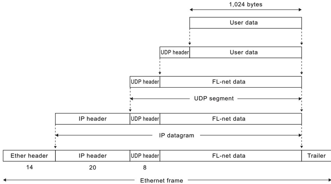
Next, the following shows FL-net data (of one frame) that can be observed on communication lines. In this example, 128-byte cyclic data is transferred.
