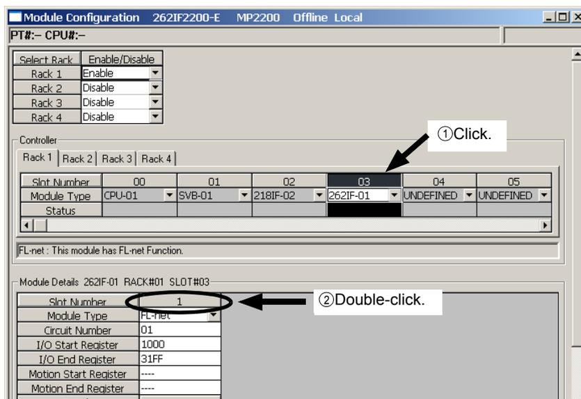
In Online Mode, the FL-net transmission definitions data saved in the Machine Controller are displayed. In Offline Mode, the definitions data saved in the personal computer on which MPE720 is running is displayed.
