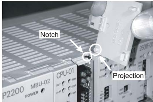
Hold the battery cover as shown in the following figure and use it to gently pull back on the Module, rotating it indicated by the arrows, to disconnect the Module from the Mounting Base. The Module will move towards you.
