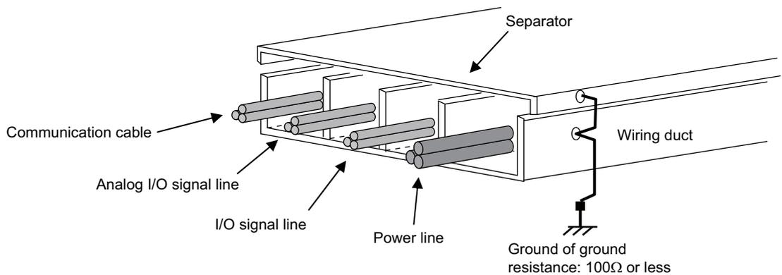
Fig. C.5 Wiring Example via a Wiring Duct
