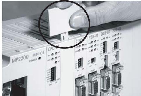
Release the hook on the bottom in the same way and remove the Option Cover.
