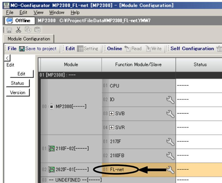
In Online Mode, the FL-net transmission definitions data saved in the Machine Controller are displayed. In Offline Mode, the definitions data saved in the personal computer on which MPE720 is running is displayed.
