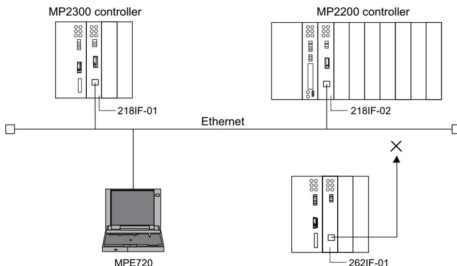
② The MPE720 engineering tool cannot be connected to the 262IF-01 directly.
