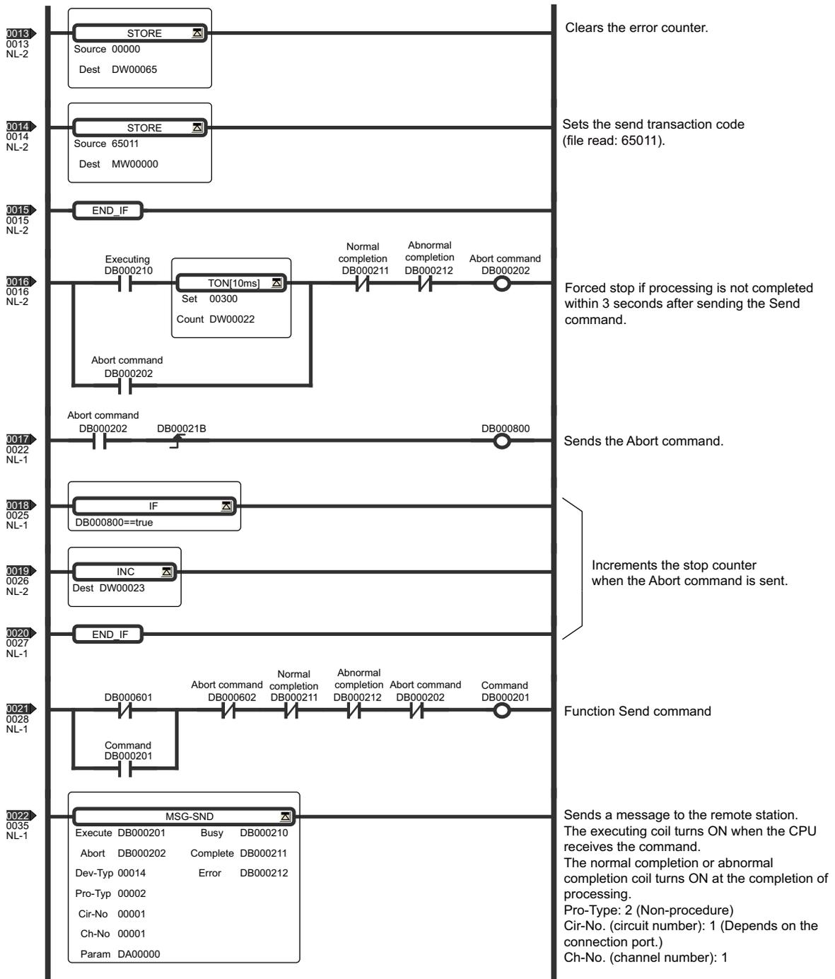
6.5.5 Sending Request/Receiving Response (Client) according to Non-procedure Protocol
