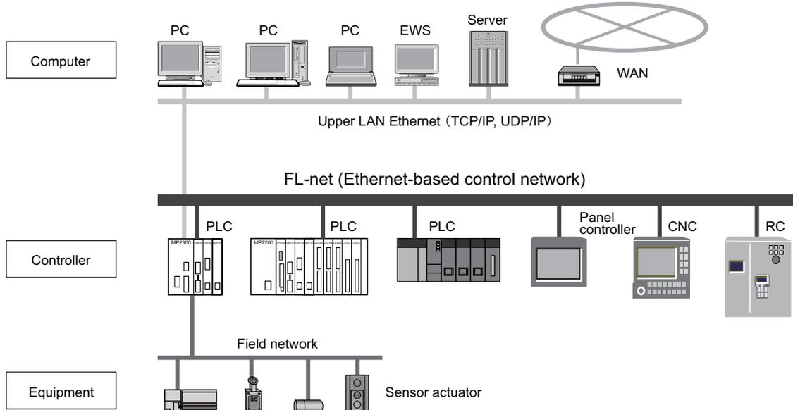
Fig. 1.1 Example of FA Control Network Configuration
