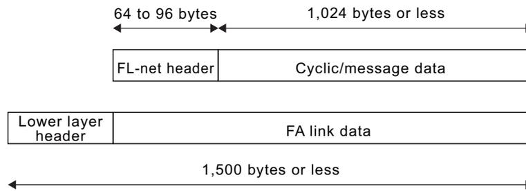
The FL-net header is put at the beginning of each frame of the FL-net protocol.
