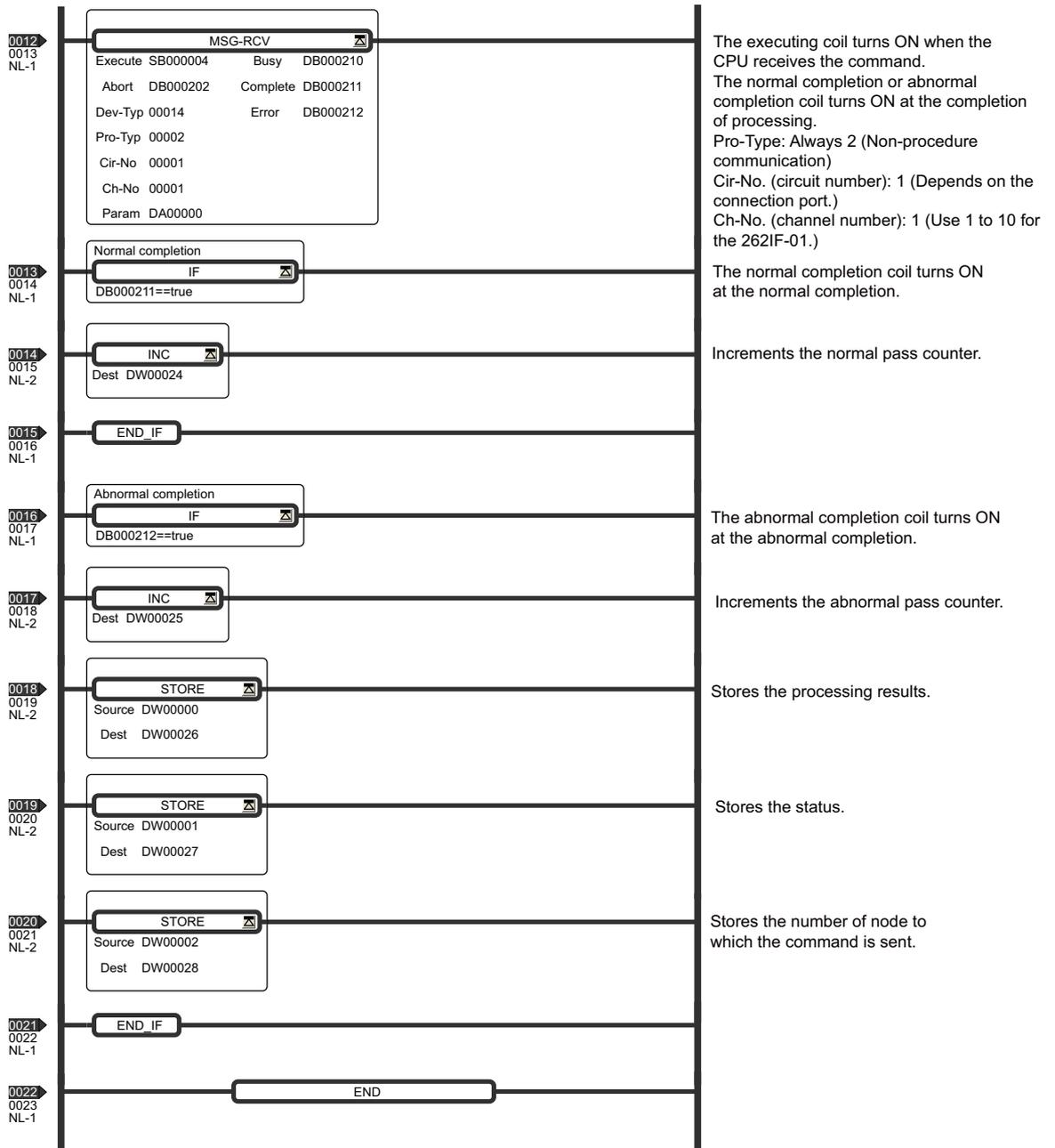
The executing coil turns ON when the CPU receives the command.
