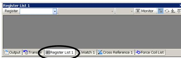
2. Enter the leading register number of the system register "MW□□□□□" (or "DW□□□□□") to be accessed in the **Register** input field and press the **ENTER** Key. The contents of the system register will be displayed starting from the leading register number.
