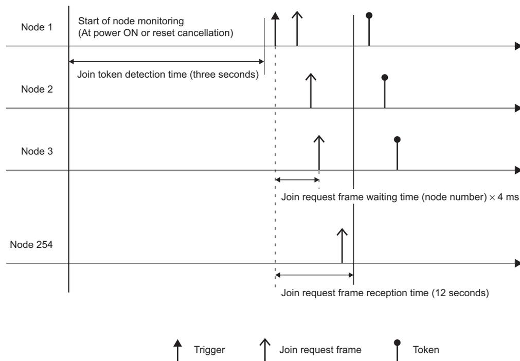
[ b ] Joining FL-net at a Halfway Point
