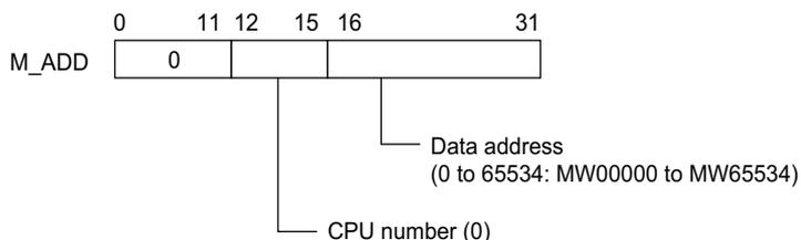
When the 262IF-01 receives the above virtual address, the 262IF-01 stores a CPU number and a data address in PARAM07 and PARAM05 respectively, and then writes to or reads from the data area shown in the following figure.
