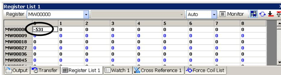
This is because a hexadecimal input value is greater than +32768 (decimal number) and it is represented as a negative value through bit inversion. In spite of negative value representation, processing is performed as a positive value.
