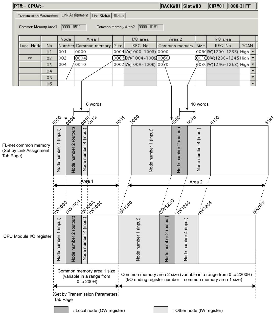
The I/O registers (IW register, OW register) are defined as a continuous area consisting of areas 1 and 2, and are filled starting with area 1. In link assignment definition, it is allowed to define only area 1 or area 2.
