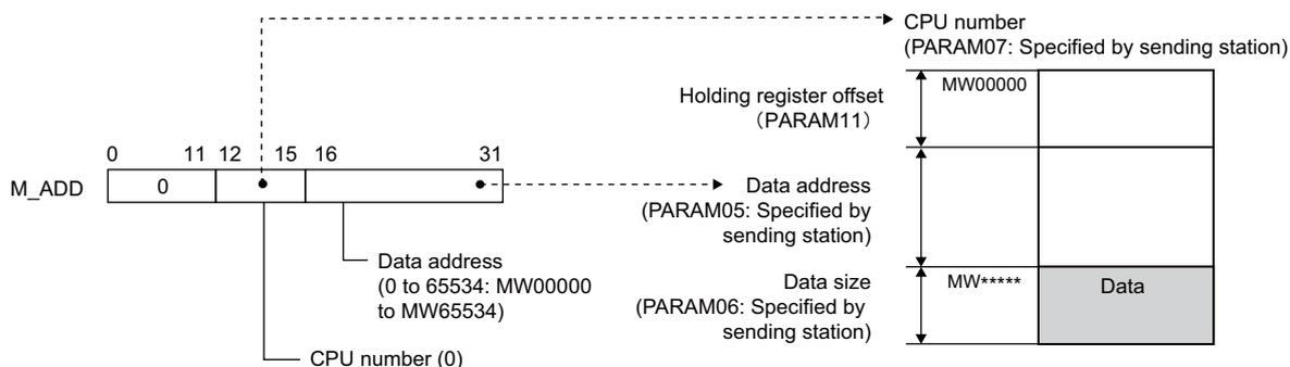
■ When the Message Is Received under Pro-Typ=2 (Non-procedure Protocol)
