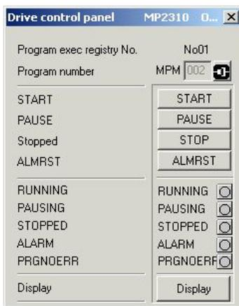
Note: The **Drive control panel** does not have the break point setting or step-by-step execution (single block execution) functions that the debug function has.
