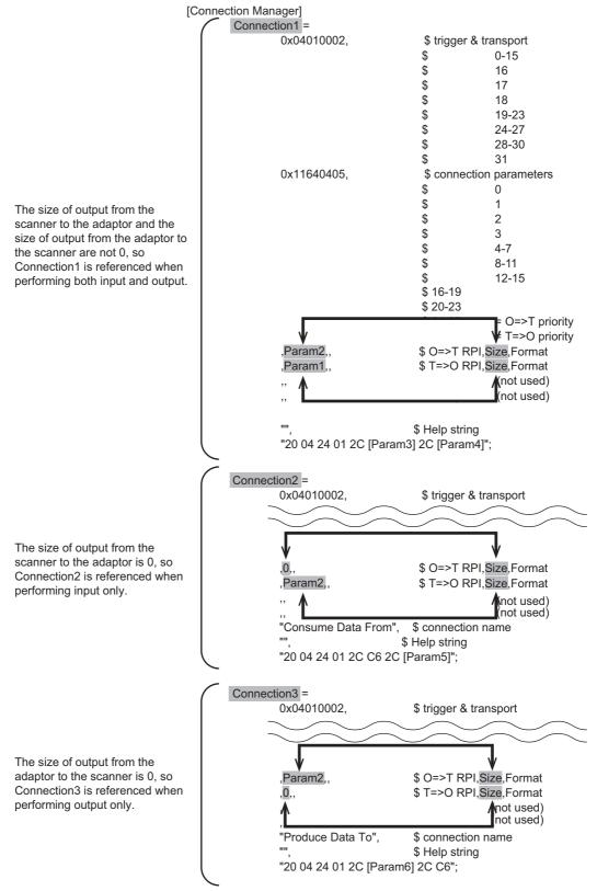
· Revision 3 of MP2000\_263IF.eds is given here as an example of the EDS file.
