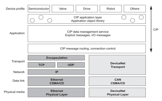
Fig. 1.1 Protocol Stack Configuration of EtherNet/IP (Includes DeviceNet)
