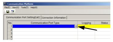
The connector on the Machine Controller side can also be connected to a computer (MPE720) using an Ethernet communication port other than that on the 263IF-01 Module. Select the communication port type according to the connector on the Machine Controller side that will be used.
