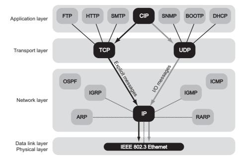
Fig. 1.2 Protocol Stack of EtherNet/IP
