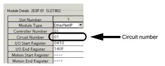
The valid range of EtherNet/IP circuit numbers is 1 to 8.
