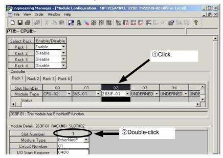
In Online Mode, the EtherNet/IP transmission definition data saved in the Machine Controller is displayed. In Offline Mode, the EtherNet/IP transmission definition data saved in the personal computer on which MPE720 is running is displayed.
