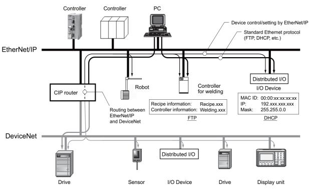
Fig. 1.3 Example of EtherNet/IP (Includes DeviceNet) System Configuration
