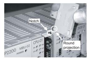
Hold the battery cover as shown in the following figure and rotate it toward the rear, using the round projection as a fulcrum to disconnect the Module from the Mounting Base connector. The Module will come out toward the front.
