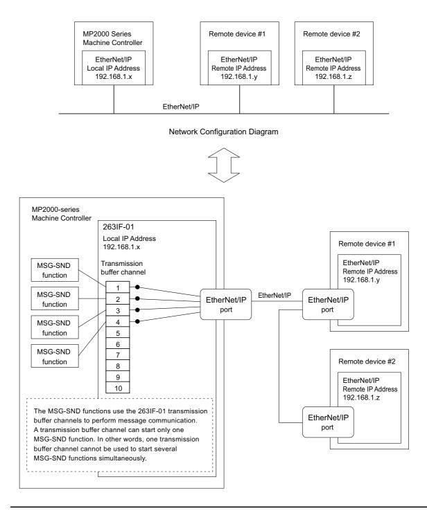
Even if different transmission buffer channels are used, it is not possible to start the MSG-SND functions simultaneously for one device (IP address). If this is attempted, an error occurs when the MSG-SND function is executed.
