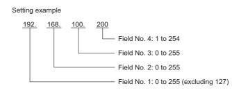
• Do not set the same address for the IP addresses and the gateway IP address.
