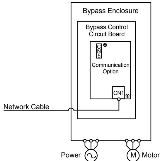
Figure 14 Option Connection Diagram (Single Port CN1 Connection)
