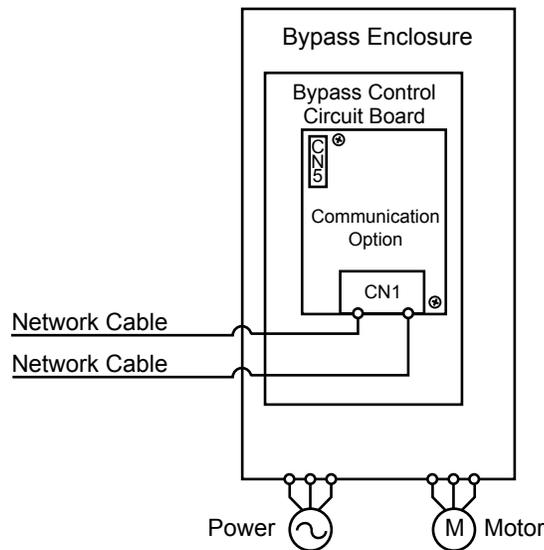
Figure 16 Option Connection Diagram (Dual-Port CN1 Connection)
