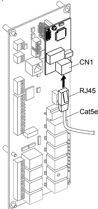
Figure 13 Connect Network Cable to Option
