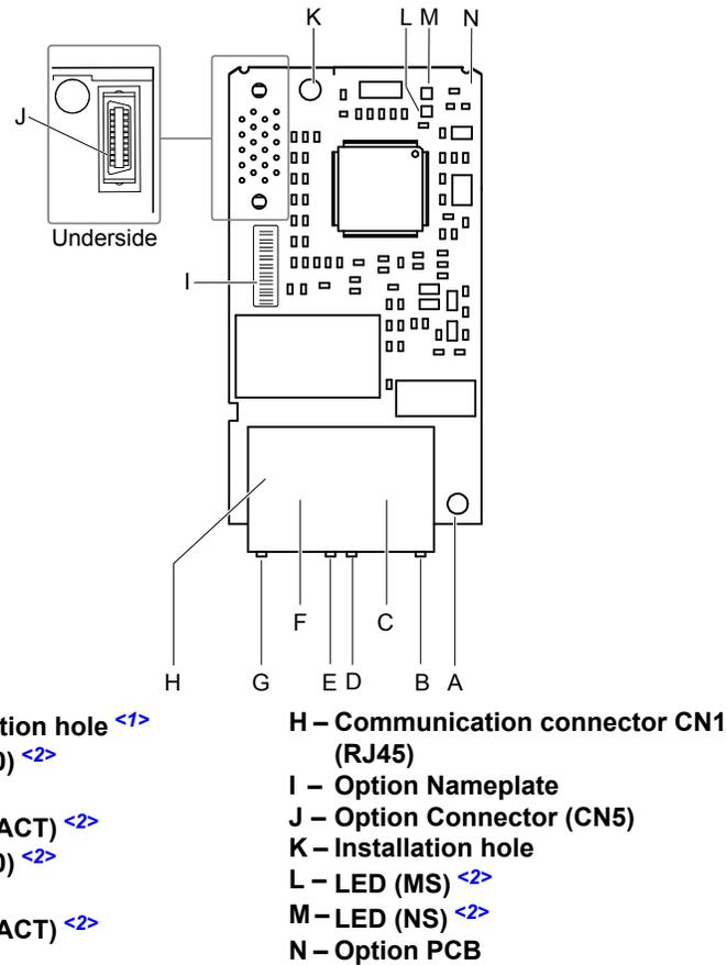
Figure 4 Option Components (Dual-Port)
