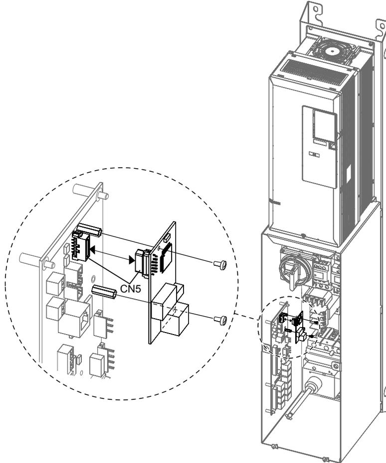
Figure 12 Insert Option into Bypass PCB CN5 Connector Port - Model Z1B1D002
