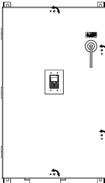
**Figure 10 Turn Front Cover Fasteners**
