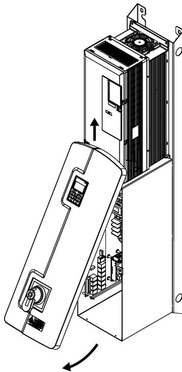
Figure 8 Lift and Remove Front Cover
