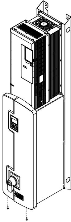
Figure 7 Remove Front Cover Screws
