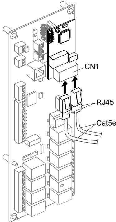
Figure 15 Connect Network Cables to Option (Dual-Port CN1 Connection)
