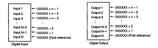
Figure 2.4 Digital VO Data Format with Bit Sequence Specification = LSB
