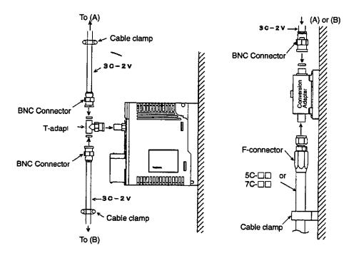
Figure 6.1 Device Connections
