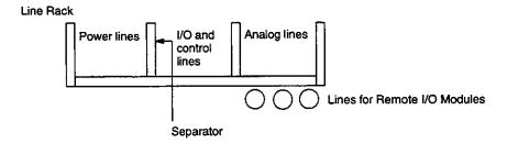
When wiring Remote I/O Module cables outside of the control panel, place them in a duct or conduit by themselves to minimize the affects of noise. Faulty operation can result if MEMOBUS lines are not sufficiently insolated.
