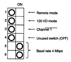
Note (1) Set the same baud rate between the Remote I/O Driver Module and Remote I/O Receiver Modules.
