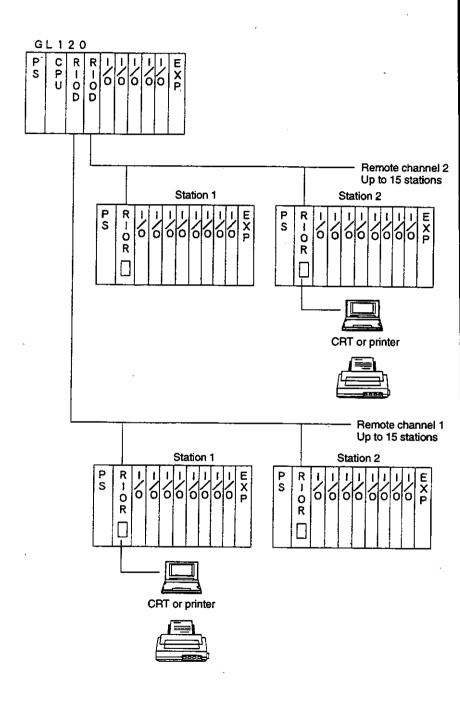
Figure 3.1 System Configuration for the COMR Instruction
