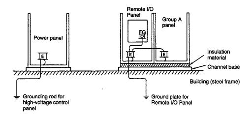
Figure 6.7 Remote I/O Panel Insulation
