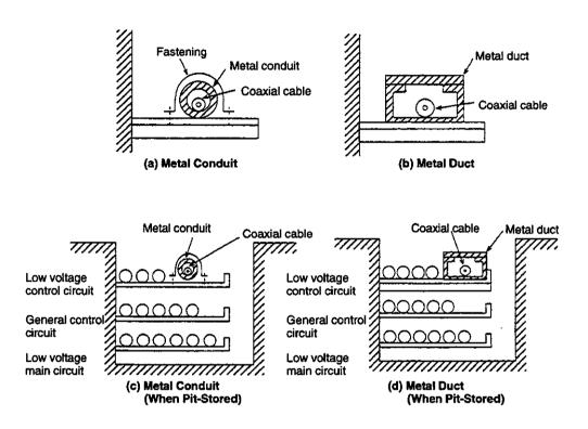
Figure 6.3 Coaxial Cable Installation
