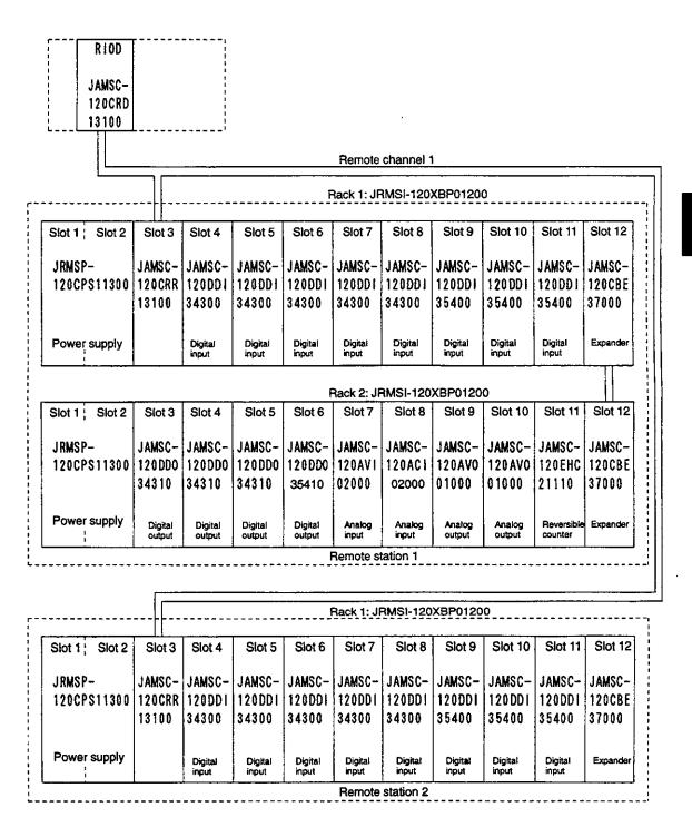
Figure 2.6 Example of I/O Module Layout
