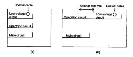
Figure 6.2 Separating Wire Ducts
