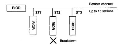
RIOD: Remote I/O Driver Module RIOR: Remote I/O Receiver Module
