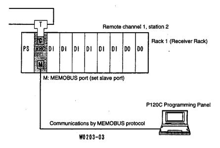
PS: Power Supply Module DO: Output Module RRC: Remote I/O Receiver Module MB: Mounting Base
