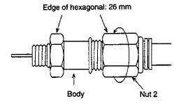
Note Fully insert the body and tighten nut 2.
