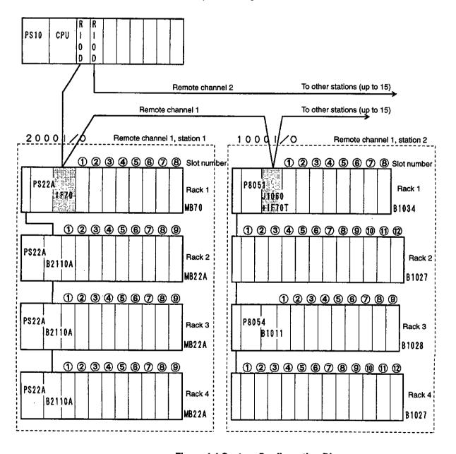
Figure 1.1 System Configuration Diagram
