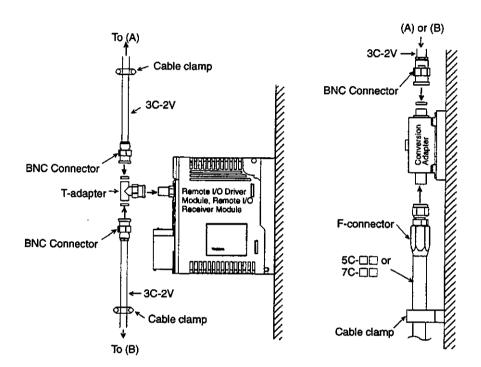
**Figure 4.1 Device Connections**
