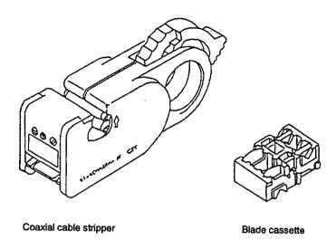
Figure A.1 Coaxial Cable Stripper and Blade Cassette
