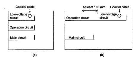
Figure 4.2 Separating Wire Ducts
