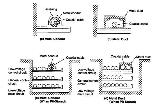
Figure 4.3 Coaxial Cable Installation
