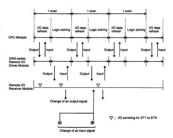
a) Change in Input Signal -> Remote I/O Receiver Module: 1 Scan or Less
