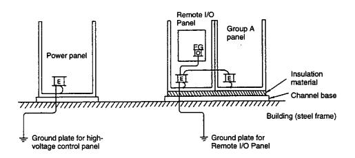
Figure 4.7 Remote I/O Panel Insulation
