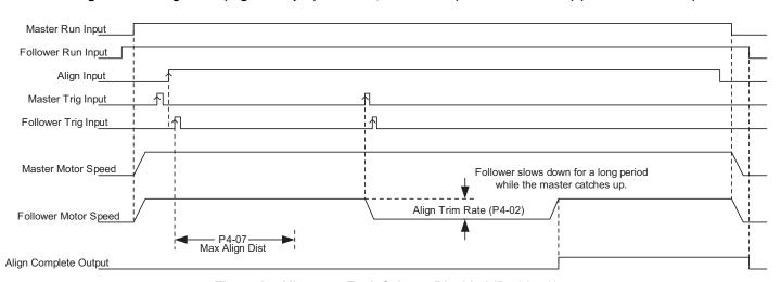
Figure 14 Alignment Fault Select = Disabled (P4-06 = 0)
