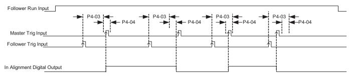
Figure 13 In Alignment (Digital Output) Function, with Offset (P4-03 = +3.00 revs) (P4-04 = 4096 cnts)
