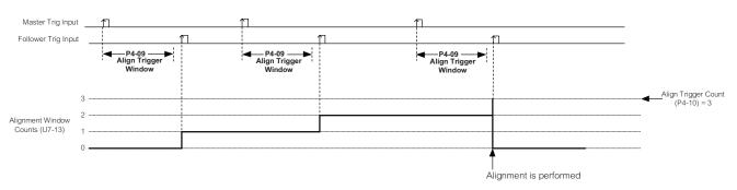
Figure 20 P4-01 = 4, Window Alignment Mode
