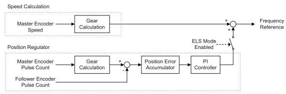
Figure 2 Simplified Block Diagram of ELS Function
