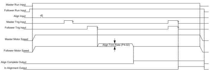
Figure 19 Normally Closed Trigger Inputs (P4-05 = 3)
