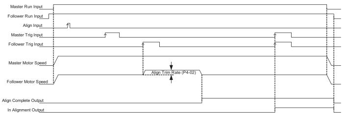
Figure 18 Normally Open Trigger Inputs (P4-05 = 0)
