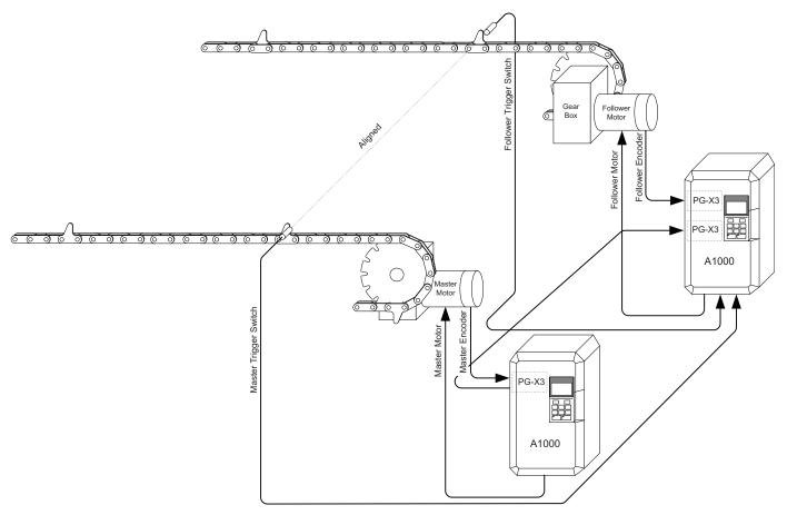
Figure 7 Simple Automation Alignment Diagram
