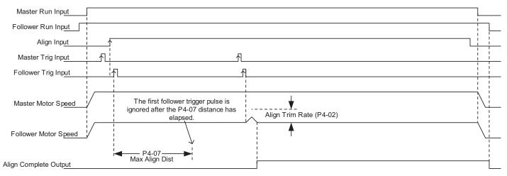
Figure 15 Alignment Fault Select = Ignore 1st Pulse (P4-06 = 1)
