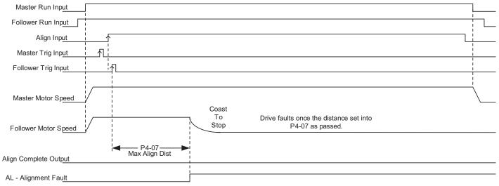
Figure 16 Alignment Fault Select = Fault (P4-06 = 2)
