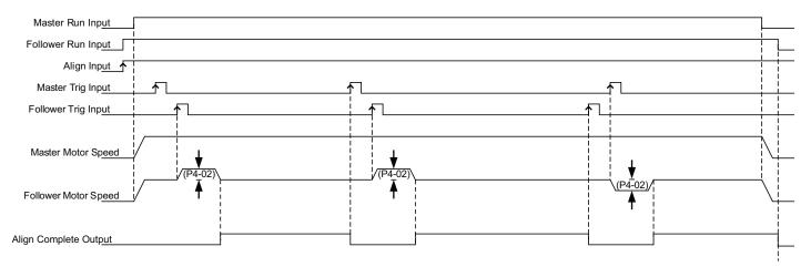
Figure 17 Continuous Alignment (P4-01 = 3)
