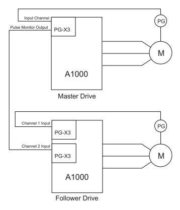
**Figure 1 Typical Configuration Connection**
