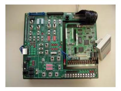
Figure 4: Simulator with G5/P5/PS5 control card installed
