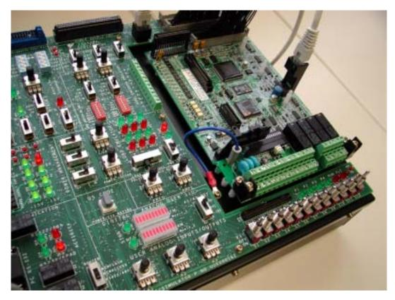
Figure 3: Simulator with E7 I/O card installed
