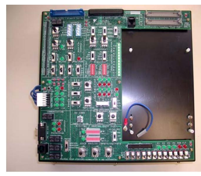
Figure 1: Simulator unit with no control card installed
