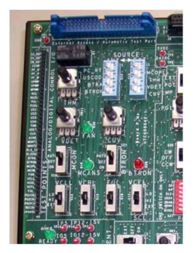
Figure 5: The test points and external access port (EAP) on the simulator
