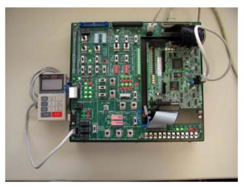
Figure 2: Simulator with G7 control card installed and running under simulated load
