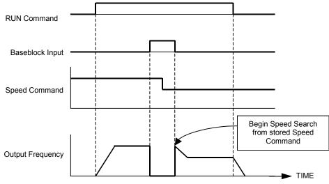
Fig. 33 External Baseblock Characteristics
