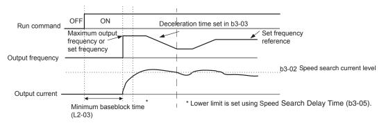
Fig. 12 Speed Search (Current Detection Method) at Startup
