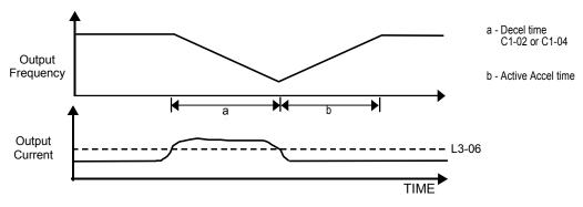
Fig. 78 Time Chart for Stall Prevention Level During Running
