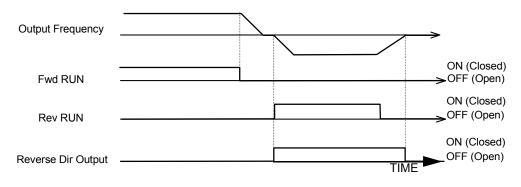
Fig. 47 Reverse Direction Timing Diagram
