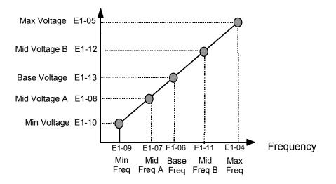
Fig. 29 Custom V/f Pattern Programming Curve
