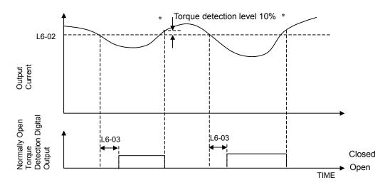
\* When the output current rises above the Torque Detection Level by approximately 10% of the Drive's rated output current the digital output is reset.
