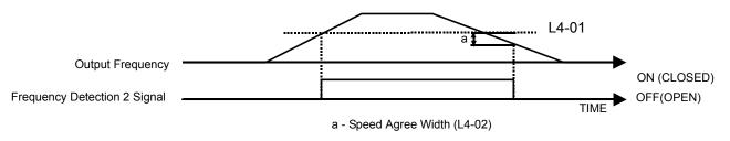
Fig. 43 Freq Detect 2 Timing Diagram
