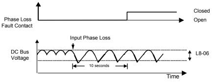
Fig. 83 Input Phase Loss Detection Diagram
