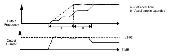
Fig. 76 Time Chart for Stall Prevention During Acceleration
