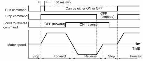
Fig. 31 3-Wire Control Timing Diagram
