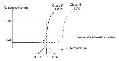
Fig. 56 PTC Thermistor Temperature-Resistance Value Characteristics
