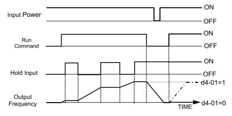
Fig. 34 Accel/Dec RampHold Function Timing Diagram
