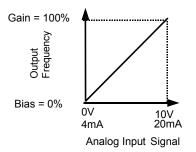
Fig. 48 Output Frequency as Commanded Via Analog Input
