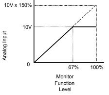
Fig. 60 Analog Output gain Setting Adjustment
