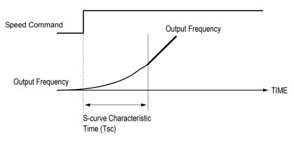
Fig. 22 S-curve Characteristic Timing Diagram
