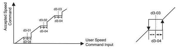
Fig. 27 Jump Frequency Characteristics
