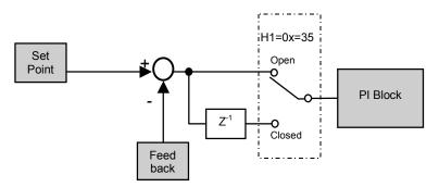
Fig. 39 PI Error signal Inversion Block Diagram
