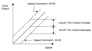
Fig. 28 Trim Control Effect on Speed Command
