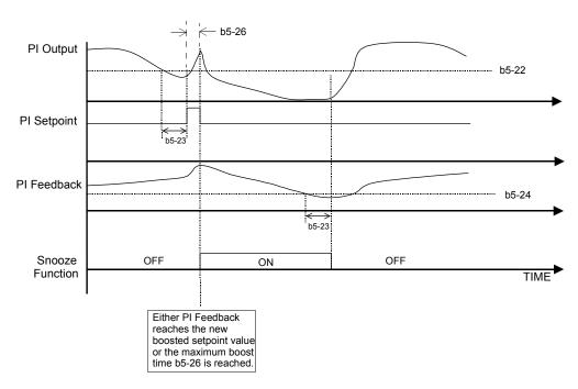
Fig. 20 Snooze Function Operation
