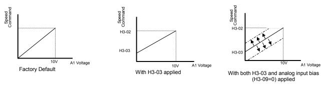
Fig. 54 Frequency Bias Applied to Analog Speed Command
