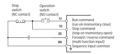
Fig. 30 Terminal Configuration for 3-Wire Control
