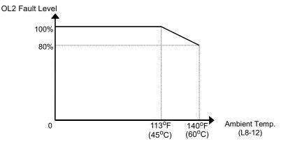
Fig. 85 Ambient Temperature Derating Curve
