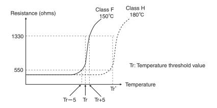
Fig. 74 PTC Thermistor Temperature-Resistance Value Characteristics
