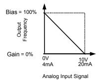
Fig. 51 Output Frequency with Inverted Gain and Bias Settings
