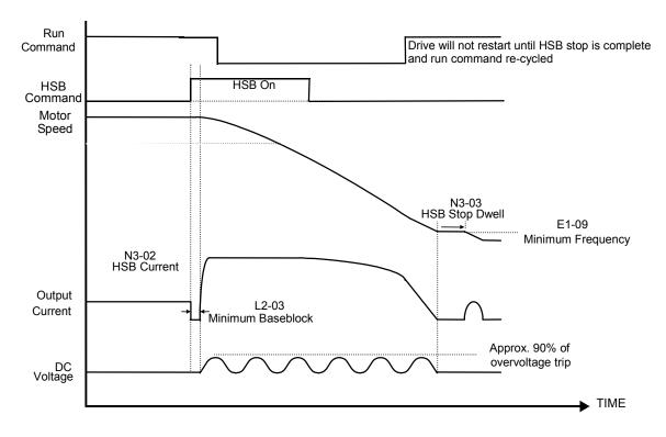
Fig. 86 High Slip Braking Timing Diagram
