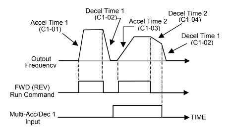
Fig. 32 Multi-Accel/Dec Timing Diagram
