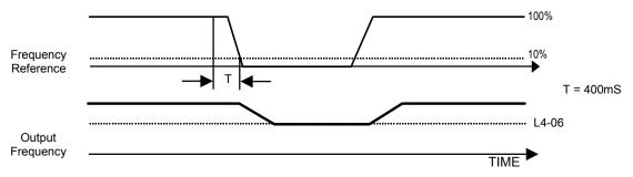
Fig. 79 Loss of Frequency Reference Timing Diagram
