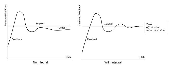
Fig. 17 PID Feedback Response Characteristics
