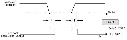
Fig. 18 Loss of PI Feedback Feature
