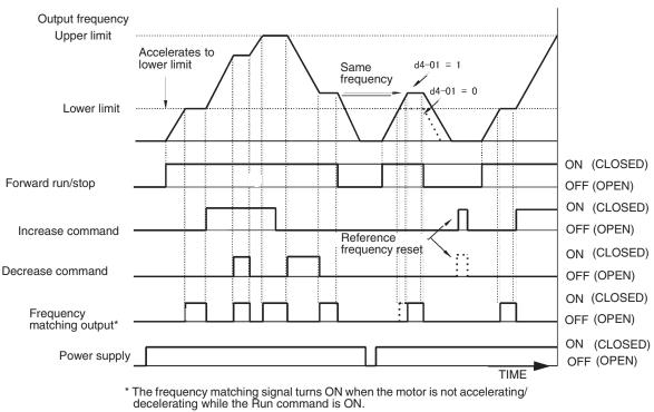
Fig. 35 Floating Point Control Time Chart
