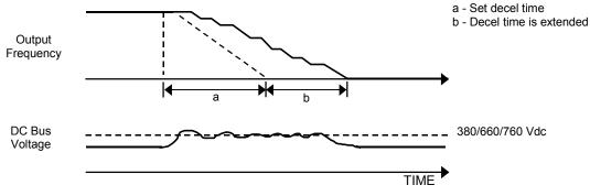
Fig. 77 Time Chart for Stall Prevention During Deceleration
