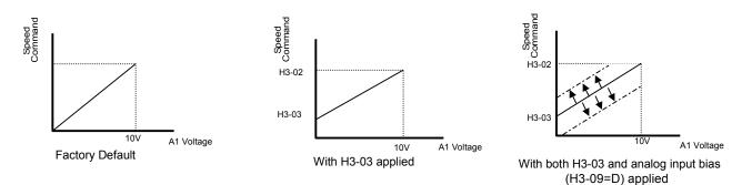
Fig. 55 Frequency Bias 2 Applied to Analog Speed Command
