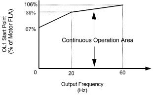
Fig. 71 Motor Overload Protection Curve
