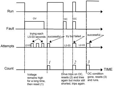
Fig. 80 Automatic Restart Timing Diagram
