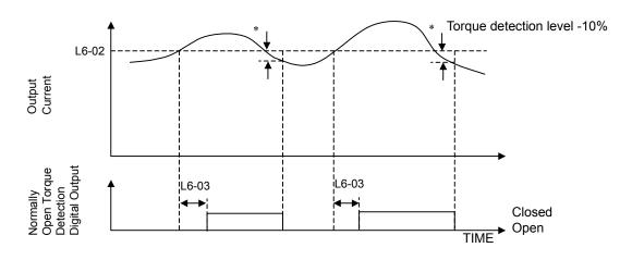
\* When the output current drops below the Torque Detection Level by approximately 10% of the Drive's rated output current the digital output is reset.
