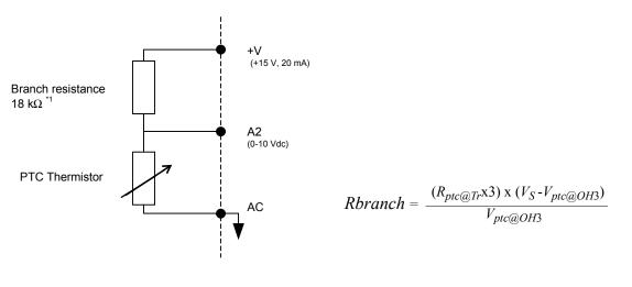
\*1 The resistance value of 18 k $\Omega$  is only valid for using a 3-phase PTC with the characteristics shown in the figure above.
