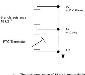
\*1 The resistance value of 18 k $\Omega$  is only valid for using a 3-phase PTC with the characteristics shown in the figure on following page.
