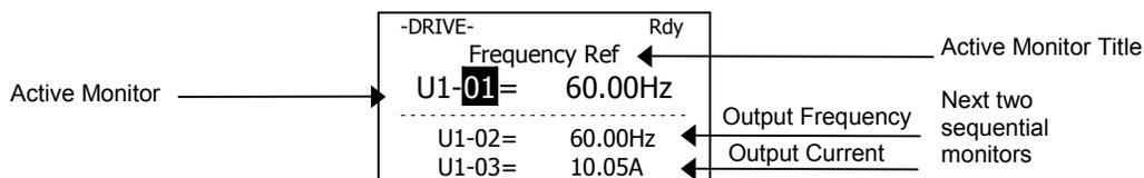
For example, if the Drive needs to display the Elapsed Timer as the Power-On monitor, then o1-01 must be set to “13” and o1-02 must be set to “4”. The next time Drive power is cycled, the digital operator displays U1-13 (Elapsed Time), U1-14 (Flash ID), and U1-15 (Term AI Level).
