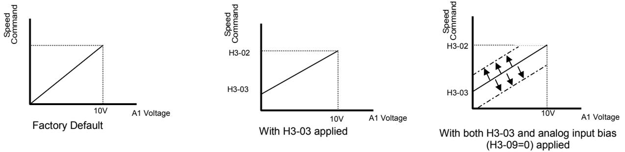
Fig. 54 Frequency Bias Applied to Analog Speed Command
