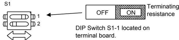
Fig. 52 DIP Switch S1
