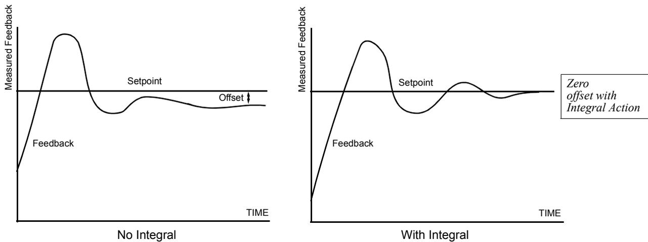
Fig. 17 PID Feedback Response Characteristics
