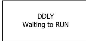
Both the ALARM and Run indicators will blink while the Drive waits to execute the Run command.
