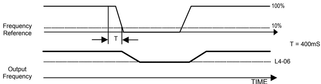
Fig. 79 Loss of Frequency Reference Timing Diagram
