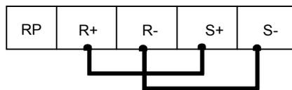
4. Turn On the terminating resistance (Move Switch 1 of Dip Switch 1 to the ON position).
