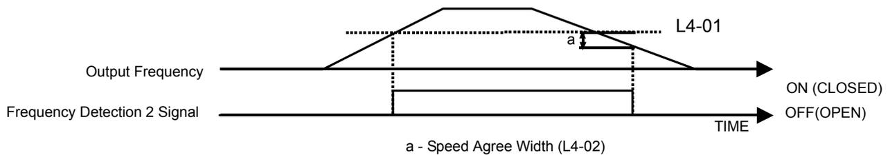
Fig. 43 Freq Detect 2 Timing Diagram
