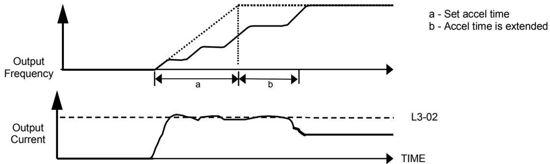
Fig. 76 Time Chart for Stall Prevention During Acceleration
