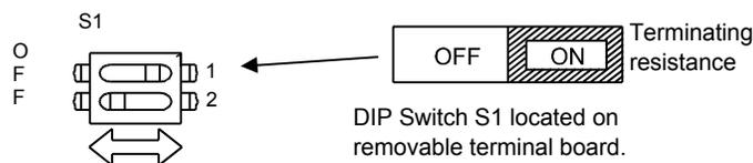
Fig. 40 DIP Switch Setting for Terminating Resistor
