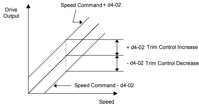
Fig. 28 Trim Control Effect on Speed Command
