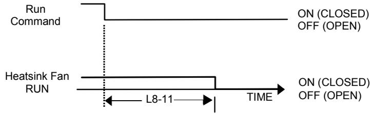
Fig. 84 Heatsink Cooling Fan Operation Timing Diagram
