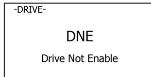
Unlike the Drive Enable digital input function (H1-0x= 6A) that requires the run command to be cycled (removed then reapplied) if the Run command was applied prior to the Drive enable input, the Run command does not need to be cycled after the Bypass Drive Enable input is closed. The Drive will run anytime both the Run and Bypass Drive Enable inputs are both closed.
