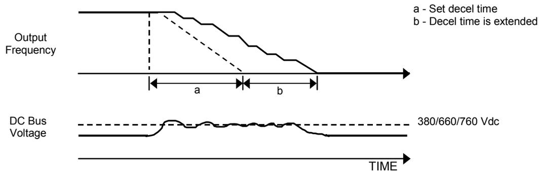
Fig. 77 Time Chart for Stall Prevention During Deceleration
