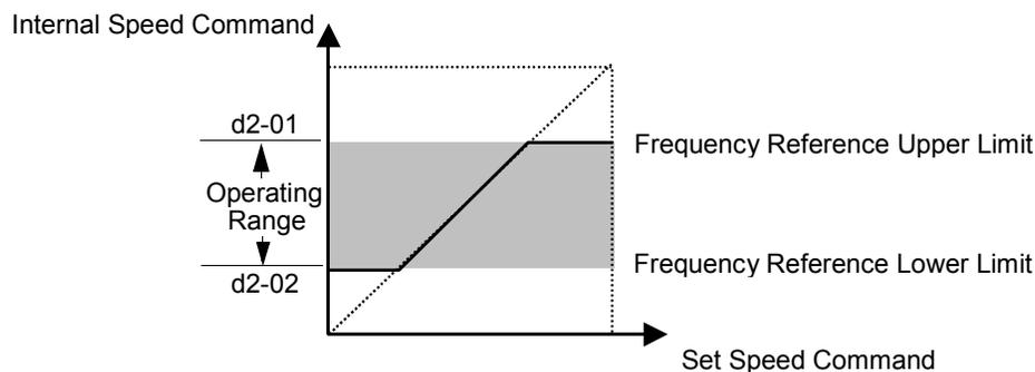
Note: See also the “Sleep” function in Figure 19 for alternate “lower limit” implementation.
