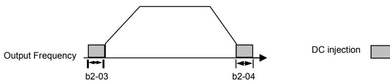
Fig. 9 DC Injection Braking During Starting and Stopping
