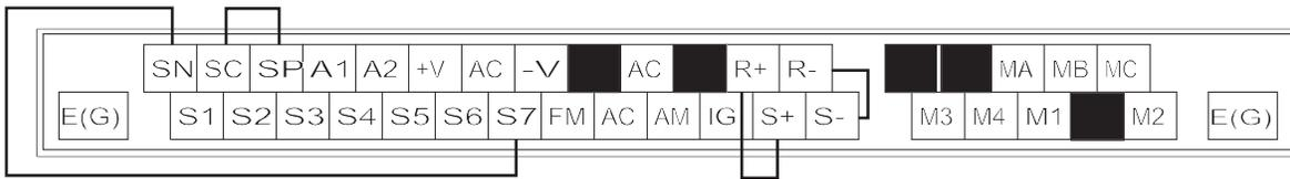
Fig. 70 Communication Terminal Connection for Self -Diagnosis Function
