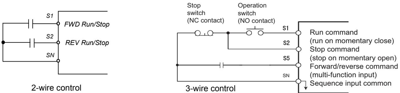
Fig. 1 2 & 3-Wire Control Wiring Examples
