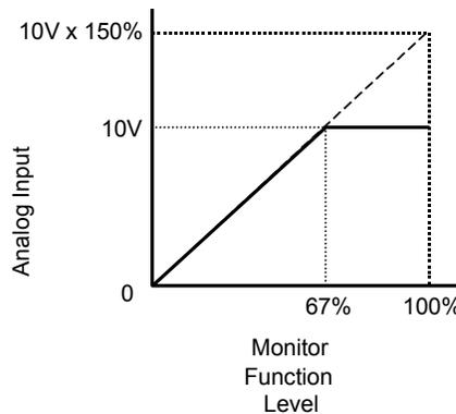
Fig. 60 Analog Output gain Setting Adjustment
