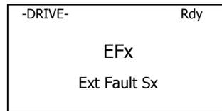
with the x in EFx and Sx represent the terminal number of the digital input that the fault was received on.
