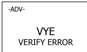
The digital operator will not display which parameters did not match, only that the verification found discrepancies in some parameter values.
