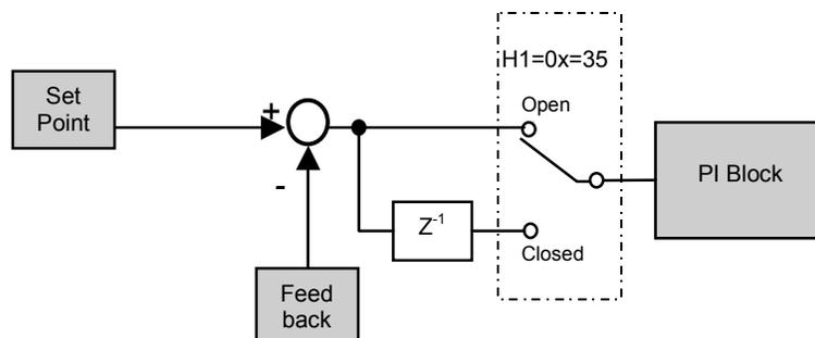
Fig. 39 PI Error signal Inversion Block Diagram
