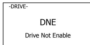
If a Run command is closed prior to the Drive Enable input being closed the Drive will not run until the Run command is cycled.
