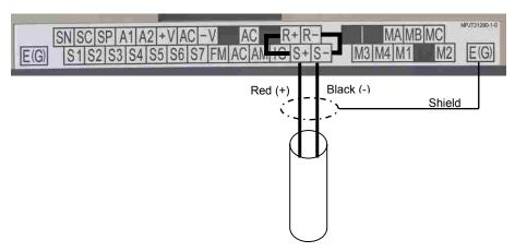
Figure A.1 - E7 Metasys N2 Network Connections
