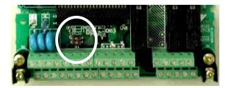
Figure A.2 – Termination Resistor Setting
