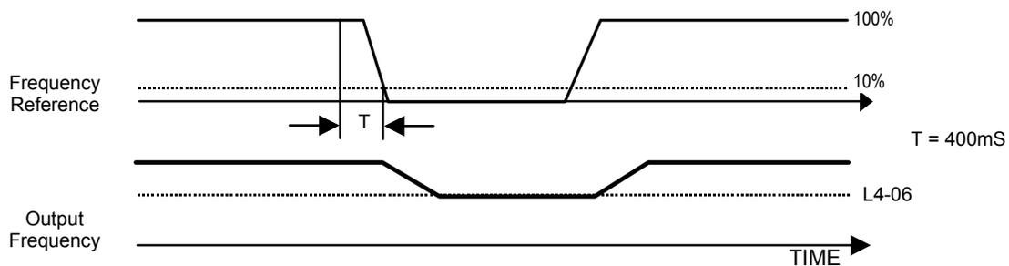
Fig 5.34 Loss of Frequency Reference Timing Diagram
