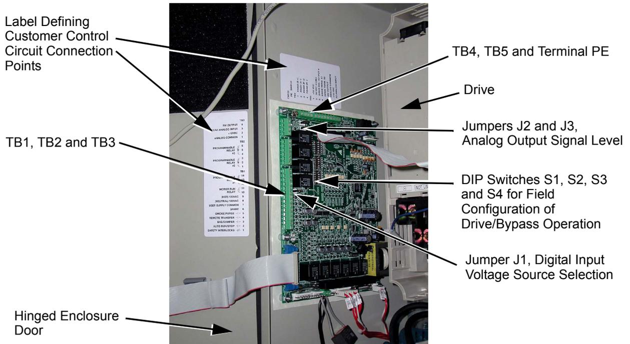
Fig 1.8 PCB A2 Control Logic and Connections
