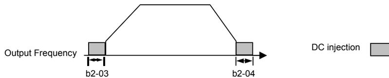
Fig 5.7 DC Injection Braking During Starting and Stopping
