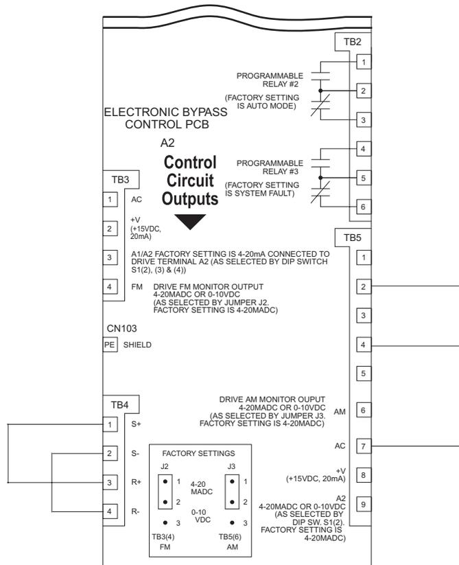
Fig. D.10 Communication Terminal Connection for Self -Diagnosis Function
