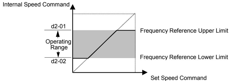
Note: See also the “Sleep” function in Figure 5.18 for alternate “lower limit” implementation.
