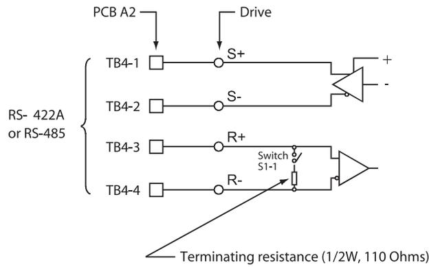
Fig 2.9 Terminating Resistor
