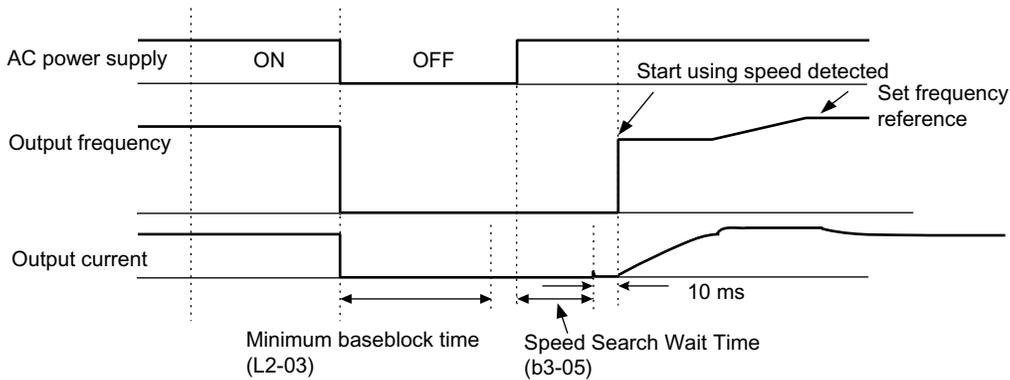
Note: If the frequency immediately before the baseblock is low or the power supply off time is long, operation may be the same as the search in case 1.
