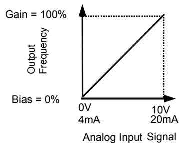
Fig 5.24 Output Frequency as Commanded Via Analog Input
