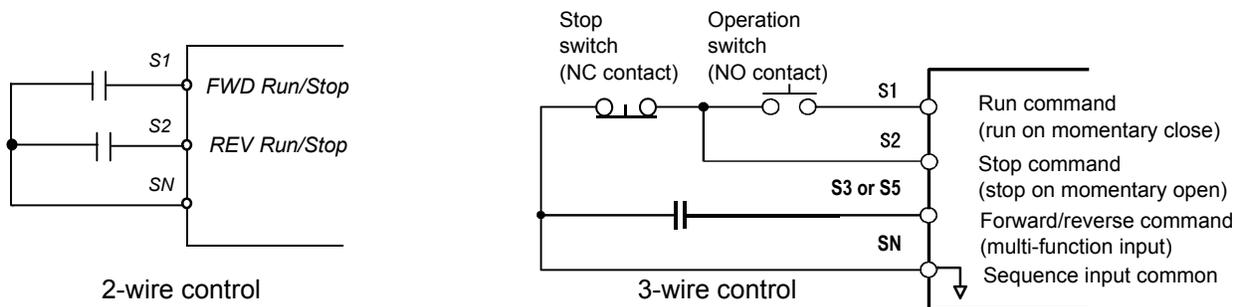
Fig 5.1 2 & 3-Wire Control Wiring Examples
