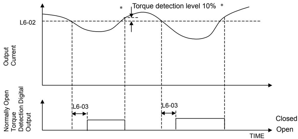
\* When the output current rises above the Torque Detection Level by approximately 10% of the Drive's rated output current the digital output is reset.
