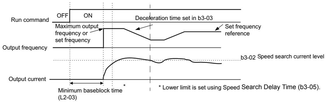
Fig 5.10 Speed Search (Current Detection Method) at Startup
