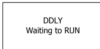
Both the ALARM and Run indicators will blink while the Drive waits to execute the Run command.
