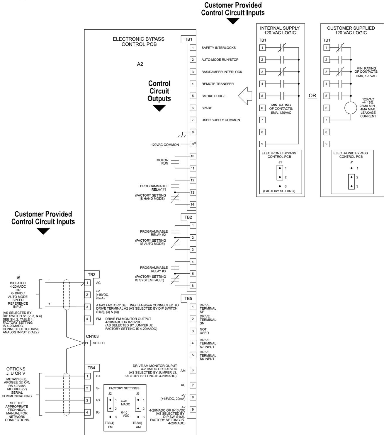
Fig 2.11 Bypass Control Circuit Inputs and Outputs
