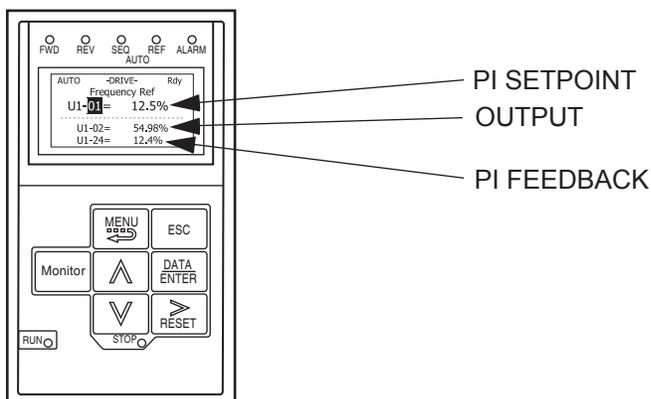
Fig 5.14 Drive Display for PI Control, AUTO Mode
