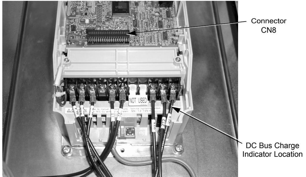
Fig 7.5 Removing the Ribbon Cable at CN8
