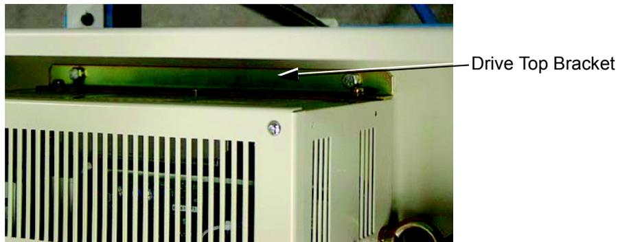
Fig 7.6 Drive Top Mounting Bracket
