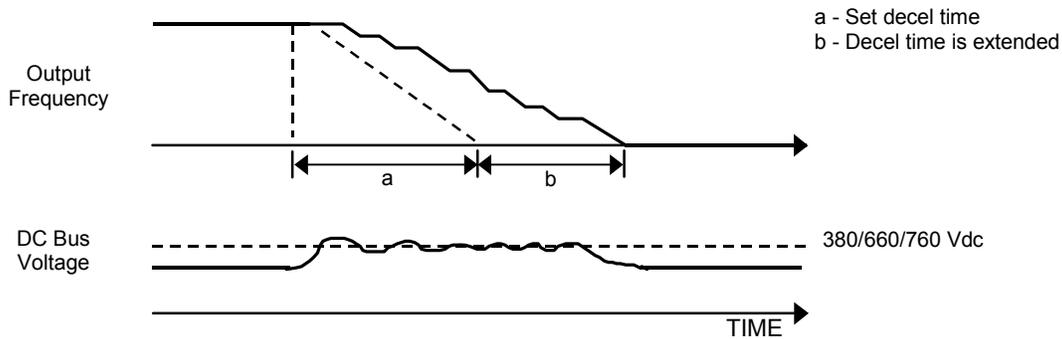
Fig 5.32 Time Chart for Stall Prevention During Deceleration
