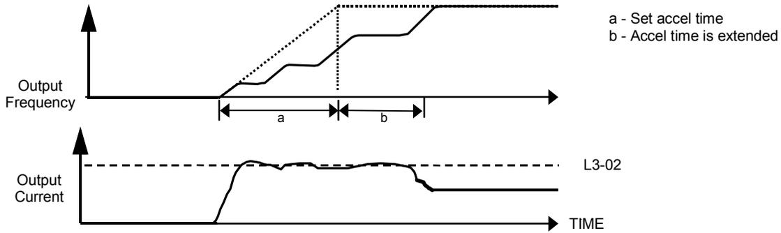
Fig 5.31 Time Chart for Stall Prevention During Acceleration
