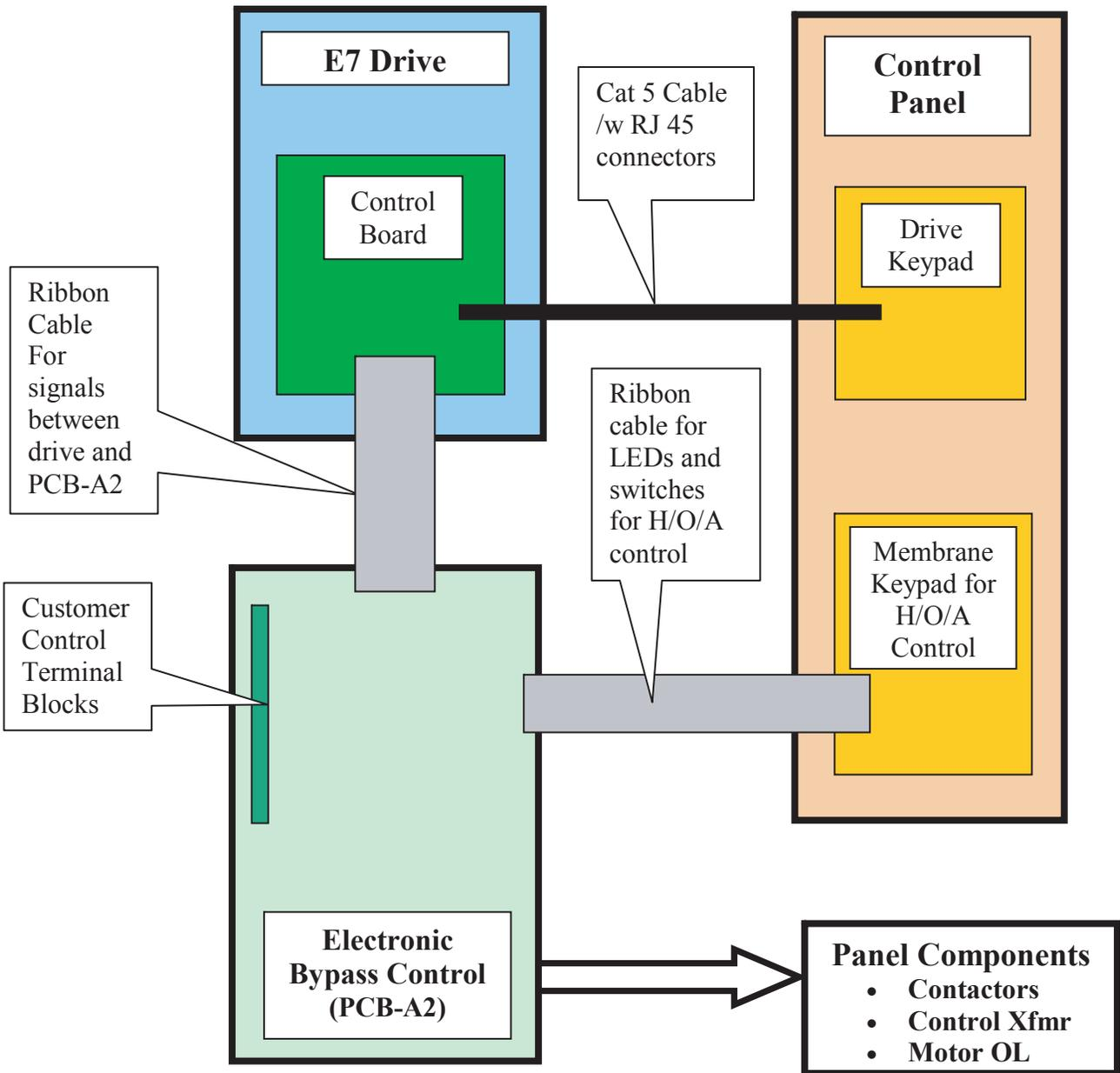
Fig 2.13 E7L Electronic Control Interconnection of Components
