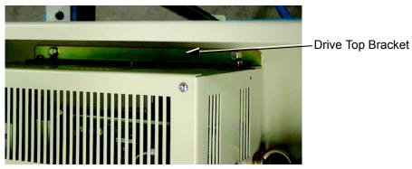
Fig 7.6 Drive Top Mounting Bracket
