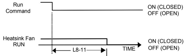
Fig 5.38 Heatsink Cooling Fan Operation Timing Diagram
