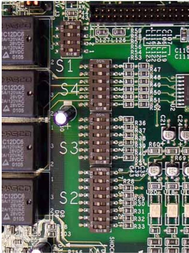
DIP Switches are “ON” when moved toward the enclosure door.
