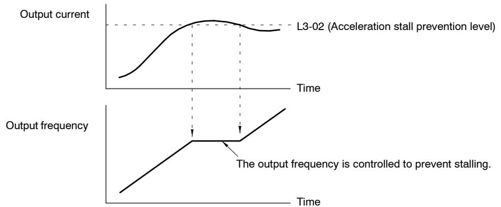
**Fig 7.43 Acceleration Stall Prevention Function: L3-01 = 1**
