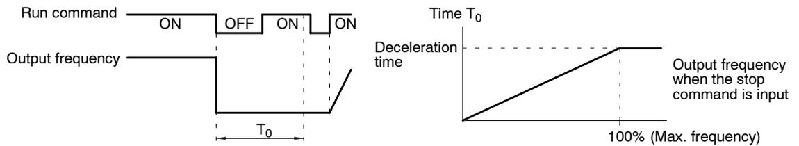
After the stop command is input, run commands are disregarded until the time  $T_0$  has elapsed. The time  $T_0$  depends upon the output frequency when the stop command is input and the deceleration time.
