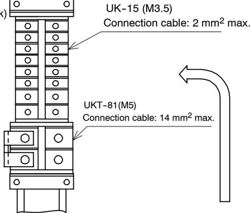
Fig 3.2 Connection Cables
