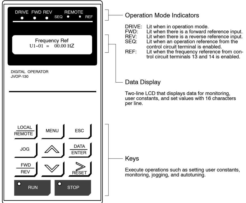
**Fig 1.3 Digital Operator Component Names and Functions**
