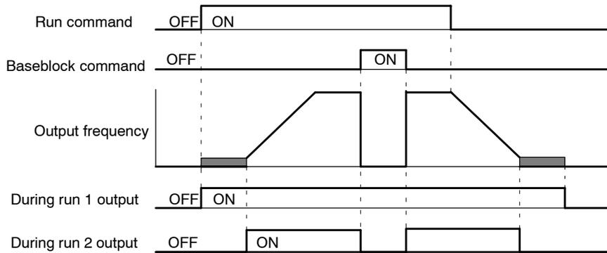
**Fig 7.39 Timing Chart for “During RUN” Output**
