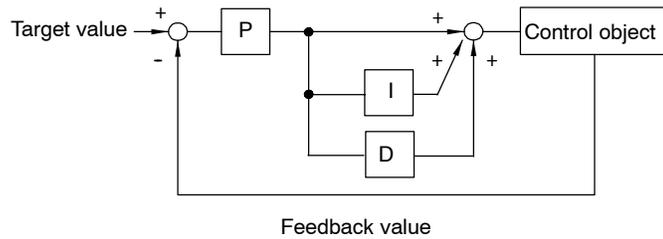
**Inverter's PID Control Function**
