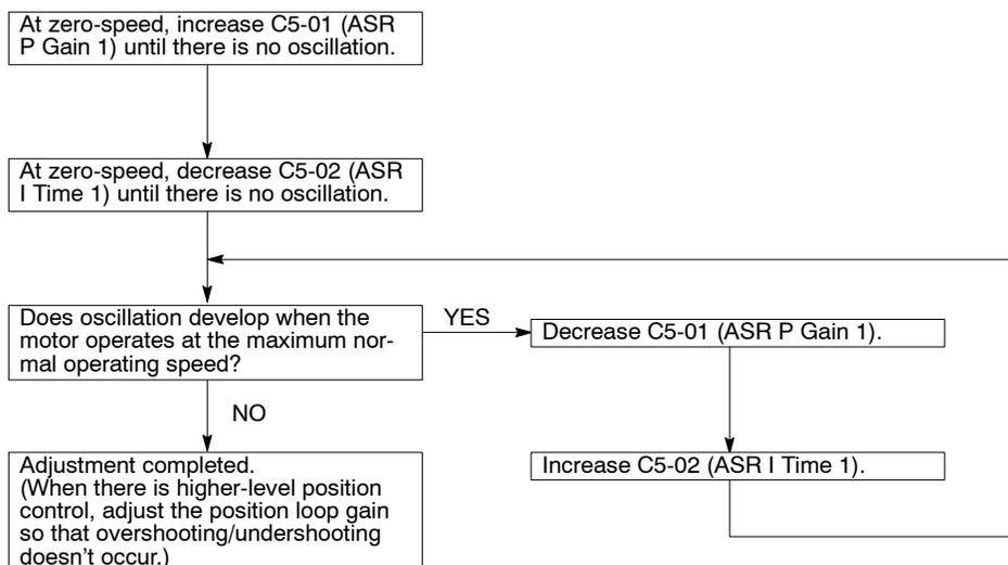
Fig 6.17 Gain Adjustment Procedure
