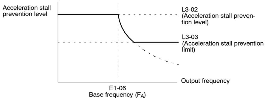
Note When the motor is used in the high-speed range, the acceleration stall prevention level is automatically lowered to provide smoother acceleration. The acceleration stall prevention limit (L3-03) limits how much the acceleration stall prevention level is lowered so that it isn't lowered any more than necessary.
