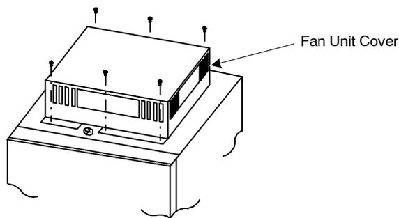
**Fig 10.2 In-panel Ventilation Fan Mounted on Ceiling**
