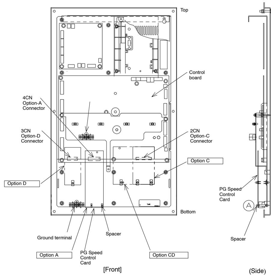
**Fig 7.29** Installing a PG Speed Control Card
