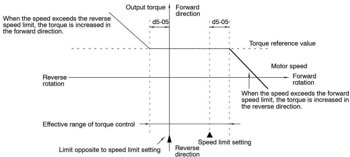
**Fig 7.11 Speed Limit Bias Settings****Operation**
