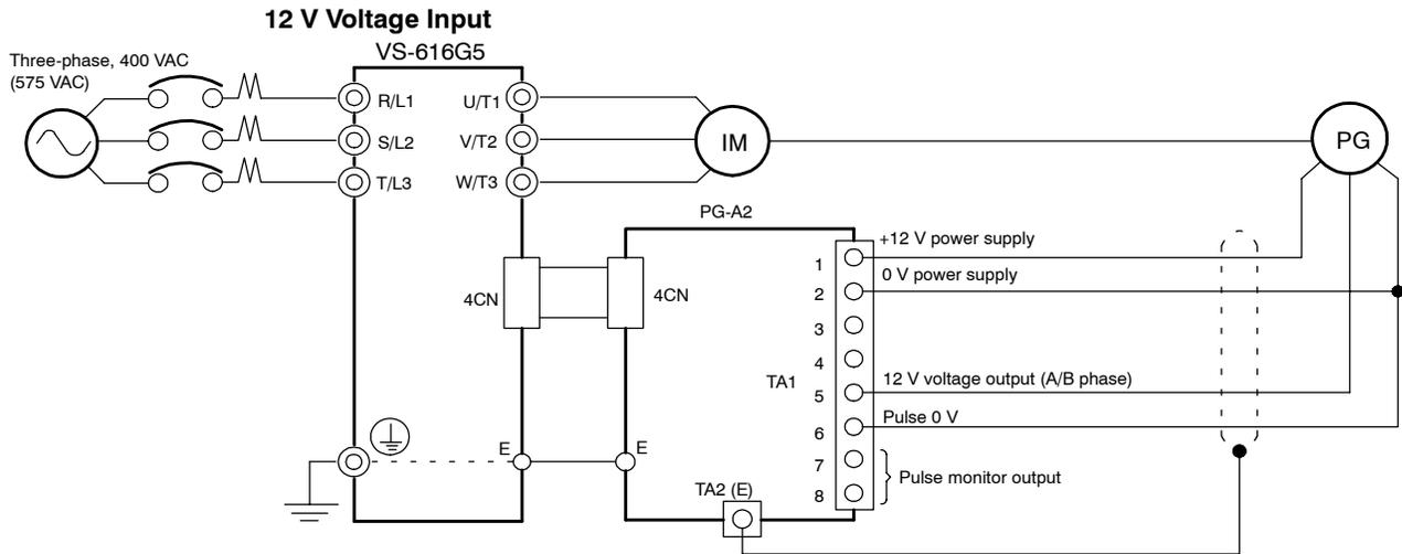
**Fig 3.9** Wiring a 12 V Voltage Input
