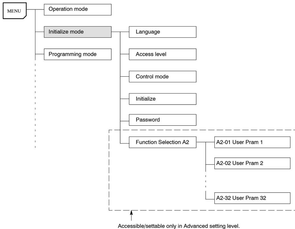
**Fig 4.7** Structure of Initialize Mode User Constants
