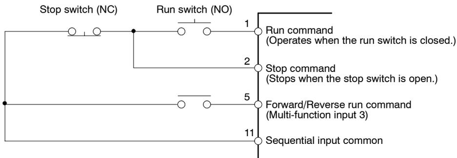
Fig 4.9 Example of Wiring for 3-wire Sequential Operation
