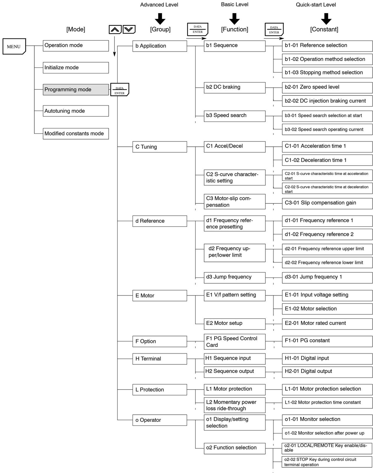
Fig 4.11 Display Structures for Different Access Levels
