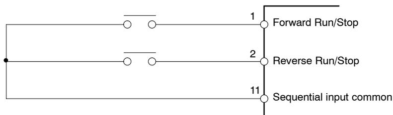
**Fig 4.8 Example of Wiring for 2-wire Sequential Operation**
