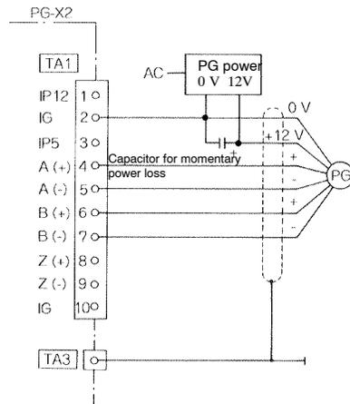
Fig 3.20 PG-X2 Connection Example
