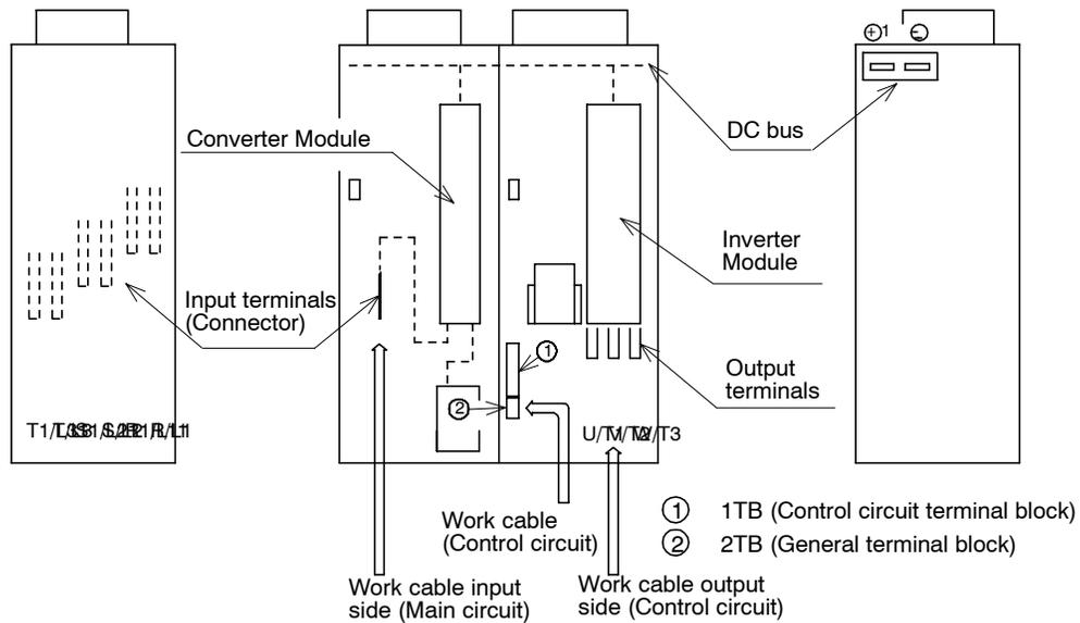
Connection cable: 325 mm<sup>2</sup> max.) (600-V CV cable, etc.)      Connection cable: 325 mm<sup>2</sup> max.) (600 V CV cable, etc.)
