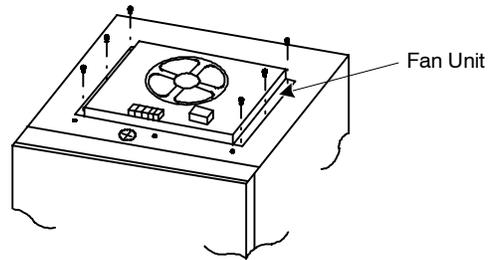
**Fig 10.3 Removal of In-panel Ventilation Fan Unit**
