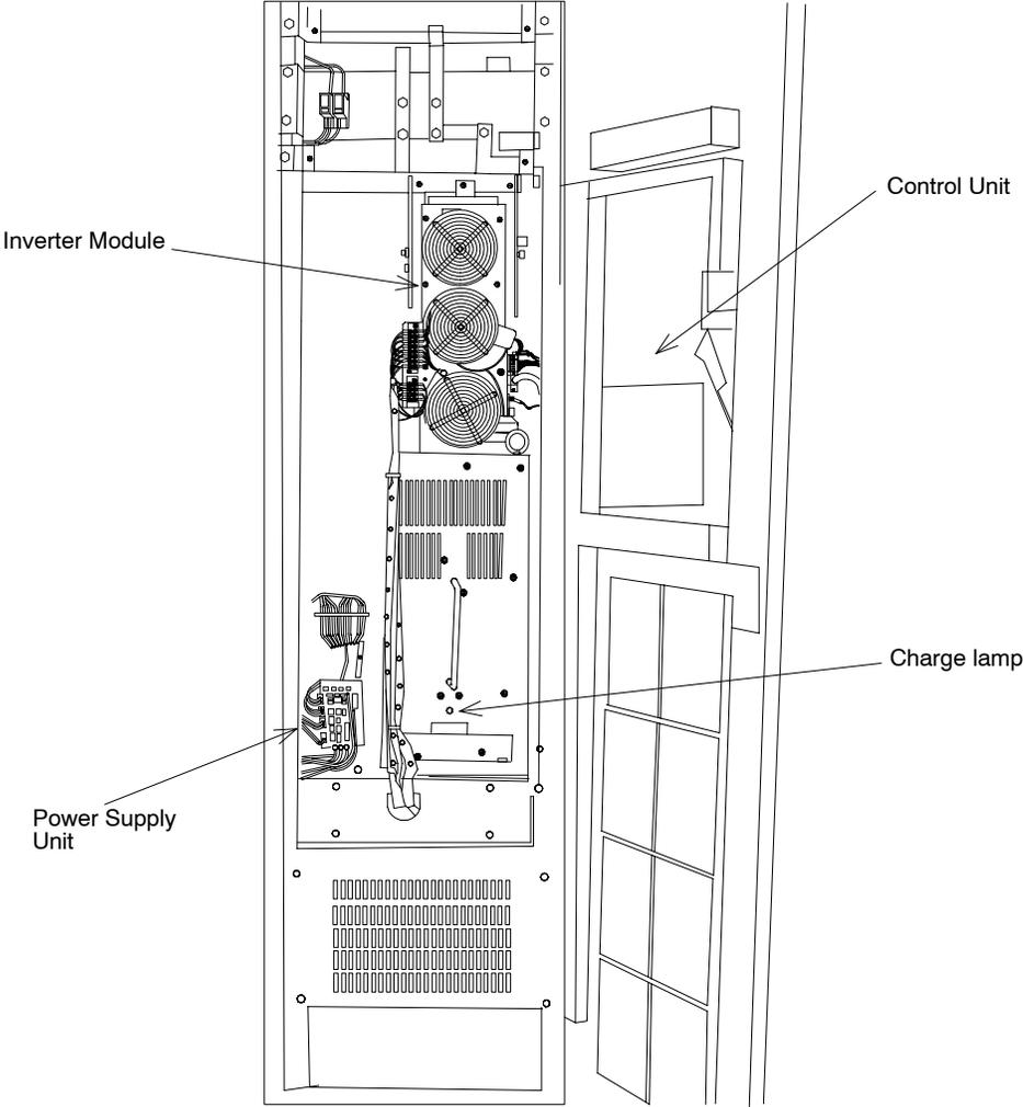
**Fig 1.2** Appearance of VS-616G5, Model CIMR-G5A (400 V, 200 kW)
