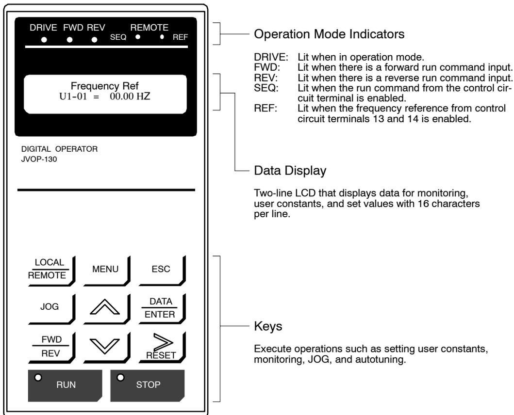
**Fig 4.1** Digital Operator Component Names and Functions
