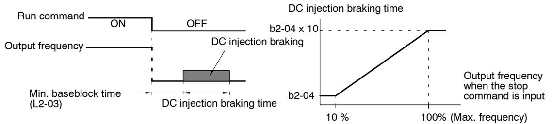
After the stop command is input and the minimum baseblock time (L2-03) has elapsed, DC injection braking is applied and the motor stopped. The DC injection braking time depends upon the output frequency when the stop command is input and the "DC injection braking time at stop" setting in b2-04, as shown in Figure 6.6.
