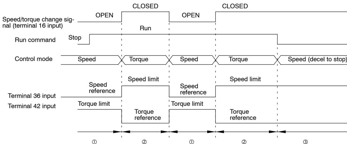
Fig 7.13 Switching between Speed and Torque Control
