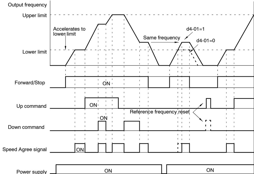
The Speed Agree signal remains ON while the run command is ON and the motor is not accelerating or decelerating.
