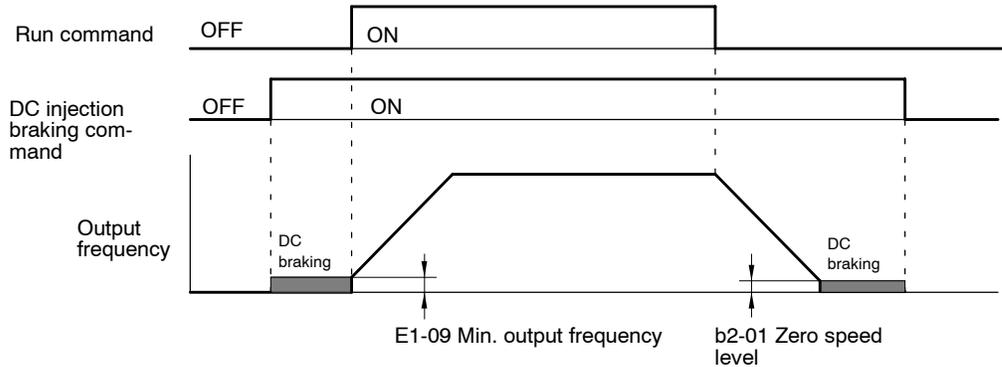
**Fig 7.37 Timing Chart for DC Injection Braking Command**
