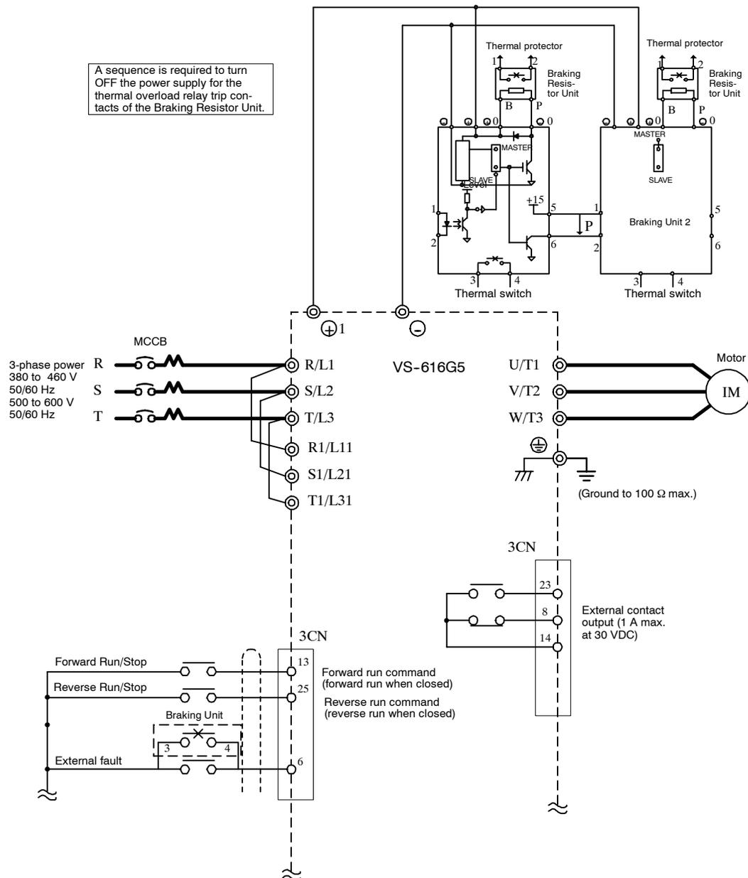
\* Disable stall prevention during deceleration by setting L3-04 to "0" when using a Braking Resistor Unit. The motor may not stop within the deceleration time if this setting is not changed.
