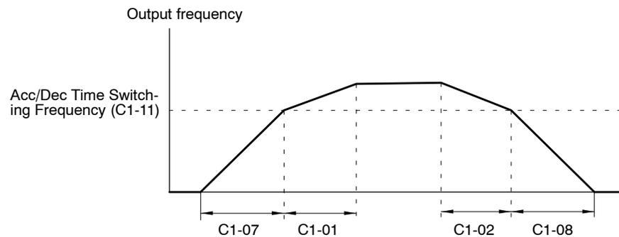
Acceleration/Deceleration Times 1 (C1-01 and C1-02) are used when the output frequency  $\geq$  C1-11
