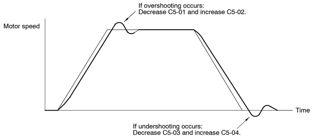
**Fig 6.24** Gain Adjustments
