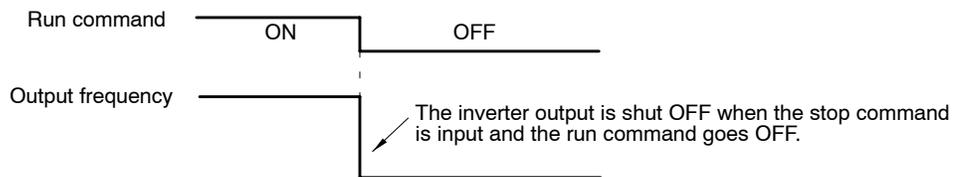
After the stop command is input, run commands are disregarded until the minimum baseblock time (L2-03) has elapsed.
