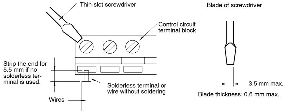
**Fig 3.17 Connecting Wires to Terminal Block**
