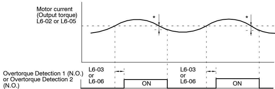
\* The overtorque detection is cleared when the current drops about 5% of the Inverter's rated current (or the motor's rated torque).
