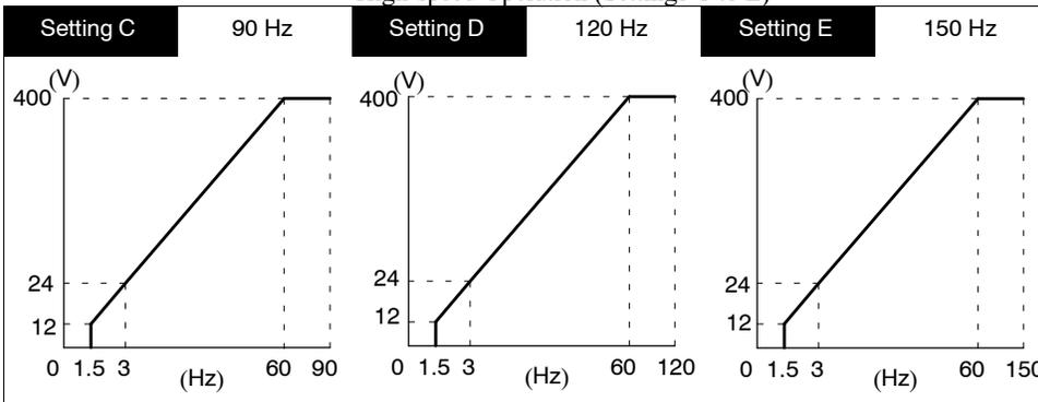
The voltages above are for 400-V Class Inverters. Multiply the voltages by approx. 1.5 for 575-V Class Inverters.
