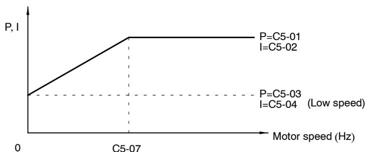
If C5-07 is set to 0.0, ASR proportional gain 1 and ASR integral time 1 are used for the proportional gain and integral time at all frequencies.
