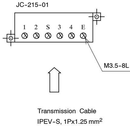
**Fig 3.3** Transmission Cable
