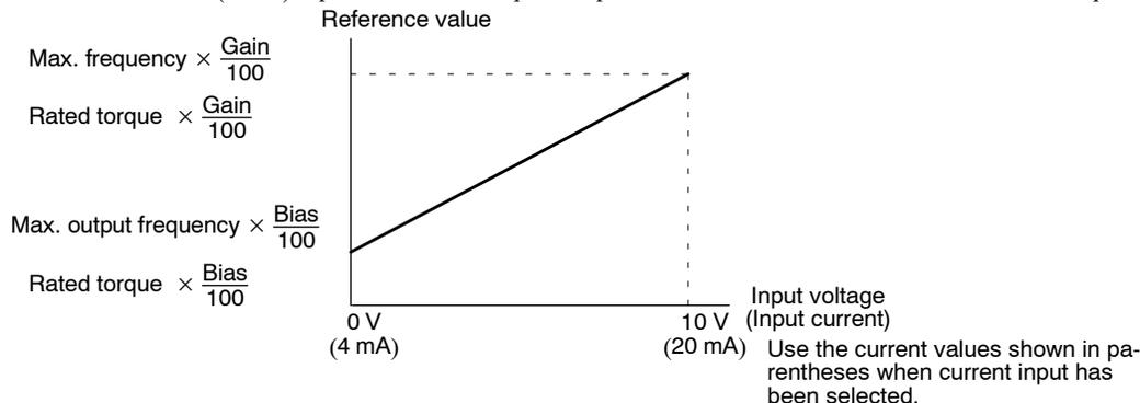
Fig 7.12 Analog Input Gain and Bias Settings
