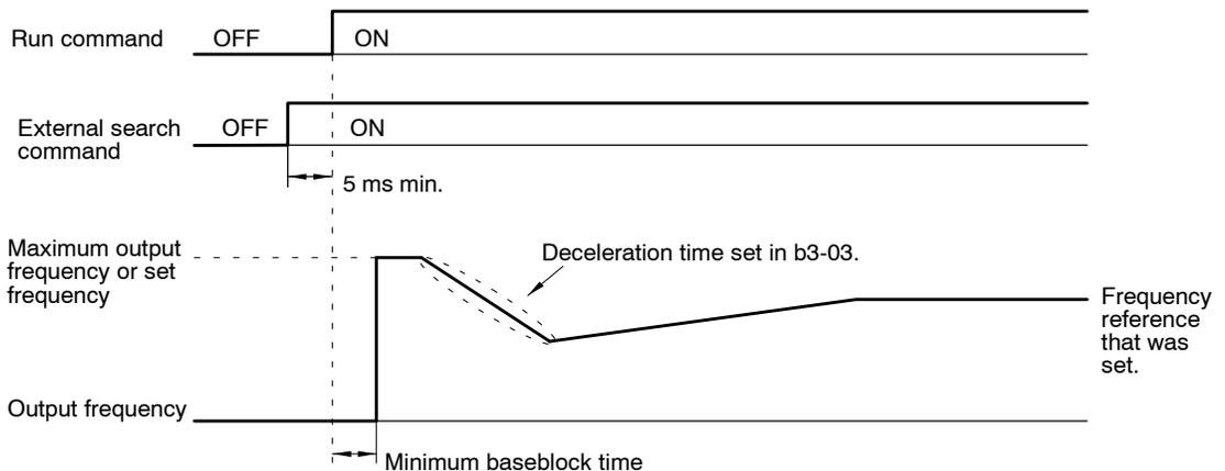
**Fig 7.38 Timing Chart for the External Search Command**
