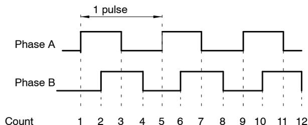
Factor of 4: By counting the rising and falling edges of phase A this method has four times the resolution of the PG.
