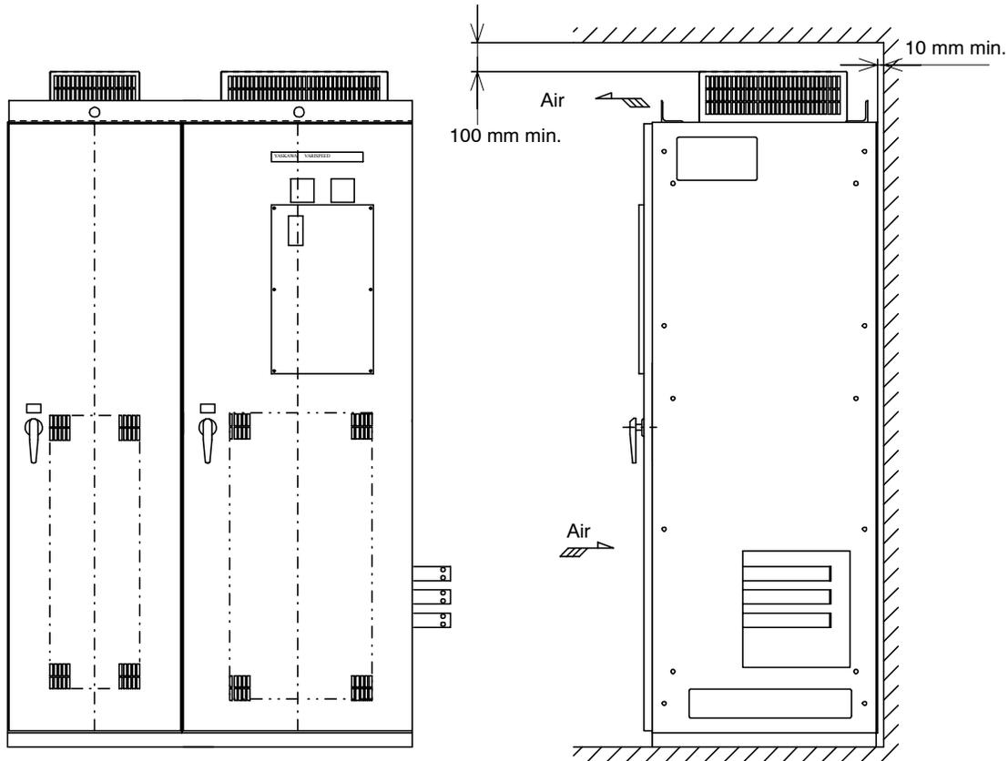
**Fig 2.9** Installation Orientation and Space for VS-616G5 Inverters
