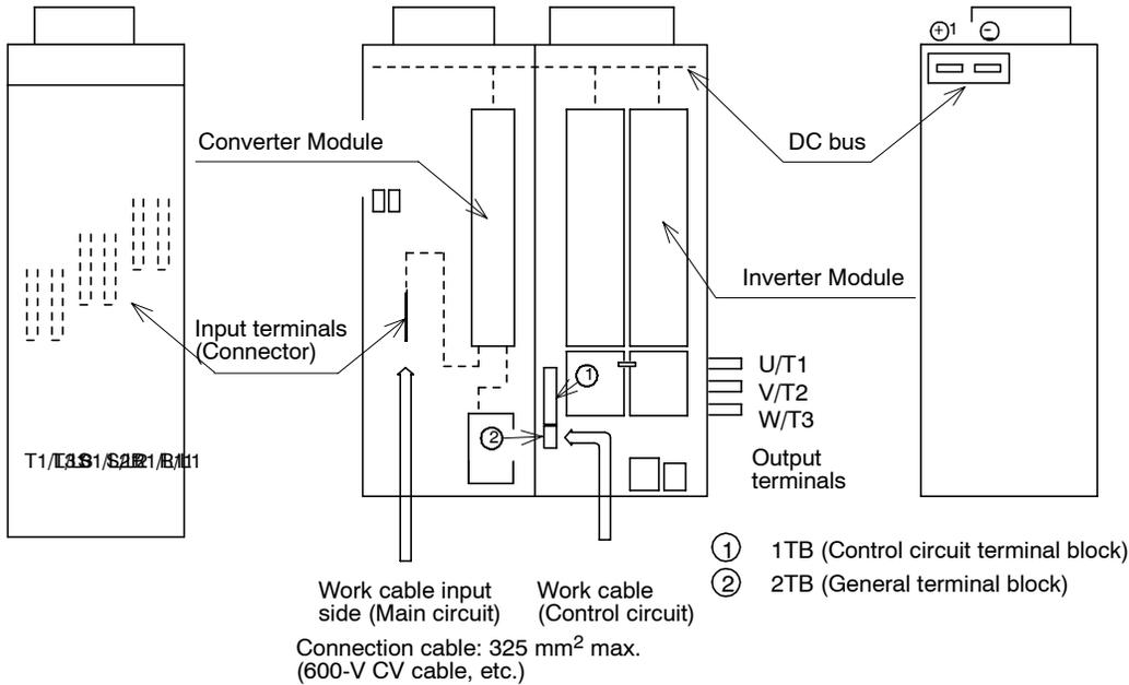
**Note** The main circuit terminals on the output side are provided as bus bar terminals on the side surface. Connections are normally made to the output terminal block on the right side.
