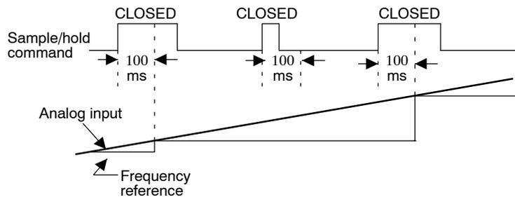
**Fig 7.34 Analog Frequency Reference Sample/Hold**
