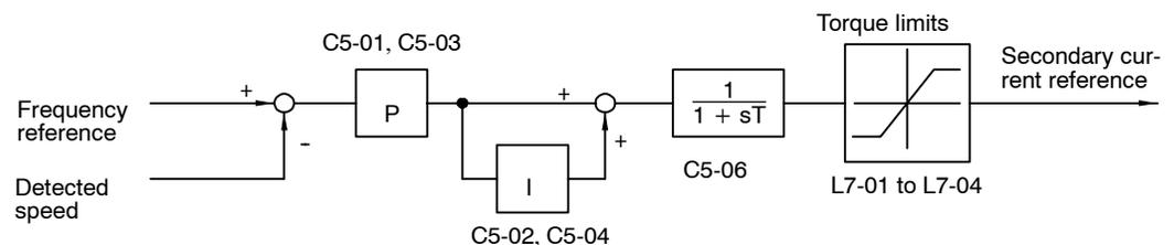
In vector flux control, the ASR's P gain is the maximum frequency standard.
