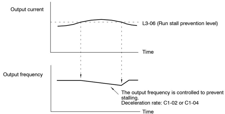
**Fig 7.46 Run Stall Prevention Function: L3-05 = 1 or 2**
