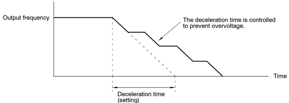
**Fig 7.45 Deceleration Stall Prevention Function: L3-04 = 1**
