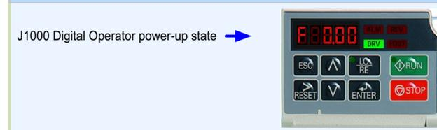
Press the **UP** key until the **FOUT** LED turns on. The display now shows the actual drive output frequency in Hz.
