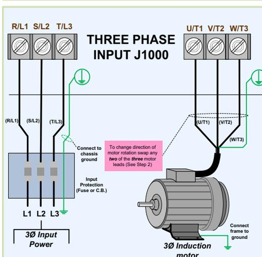
Fig. 2: Input Power and Output Motor Electrical Connections for Three Phase Input J1000
