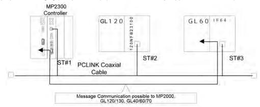
Figure 1.3 Message Transmission Between Controllers Connection Diagram
