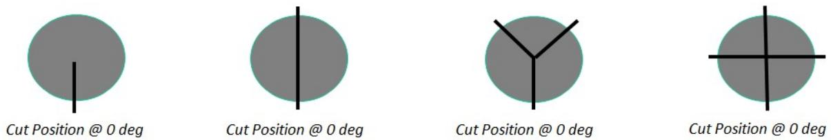
**FIGURE 4: CUT POSITIONS FOR VARIOUS KNIFE CONFIGURATIONS**
