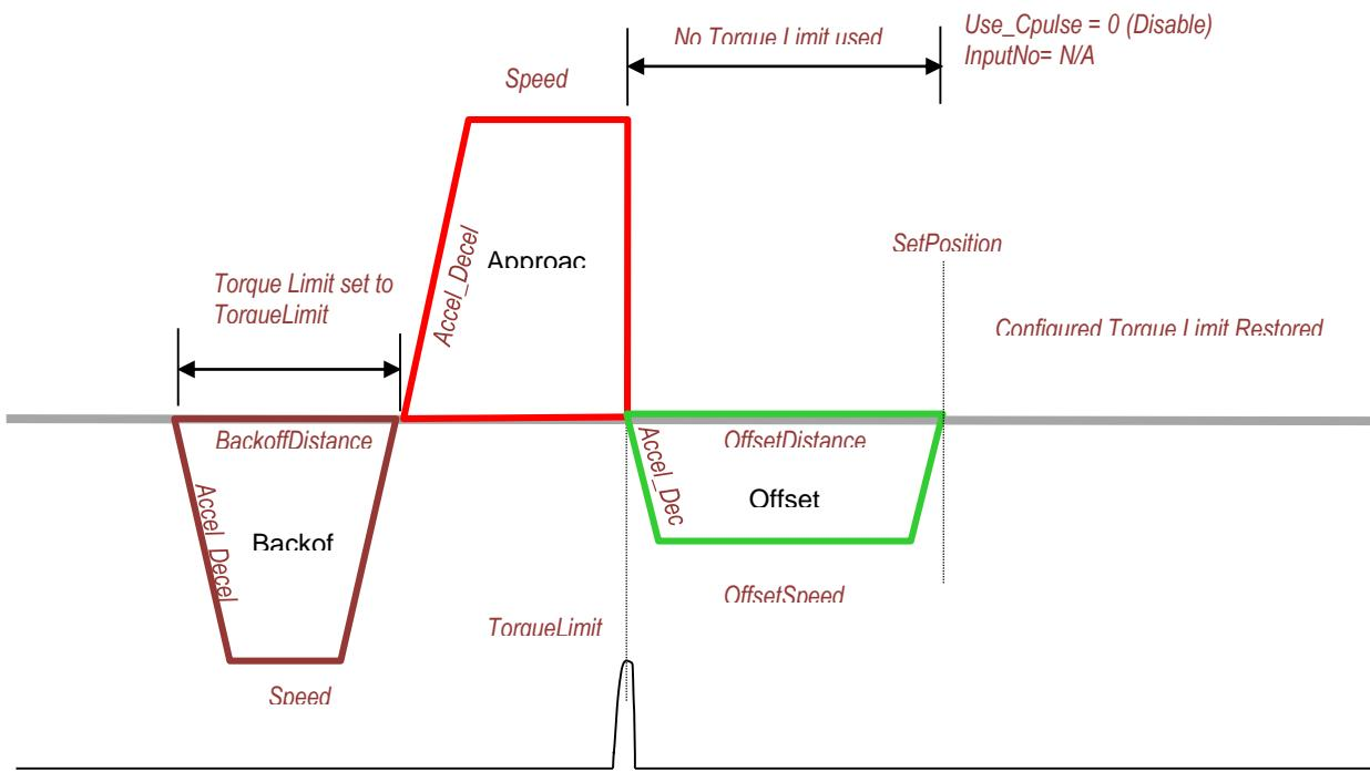
Home to Hard Stop with C-Pulse moves the servo under a Torque Limit until the hard stop is reached according to the following sequence:
