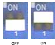
Figure C.4 – V7 PROFIBUS-DP Option Termination Settings
