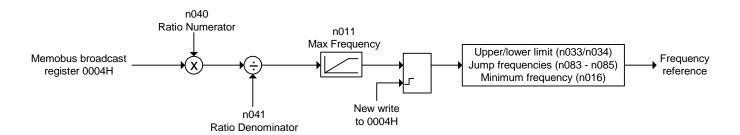
Fig. 2 – Block Diagram of Winder Ratio Frequency Reference
