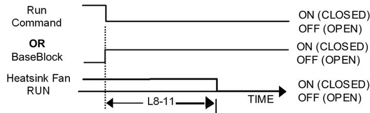
Figure 109. Heatsink Cooling Fan Operation Timing Diagram
