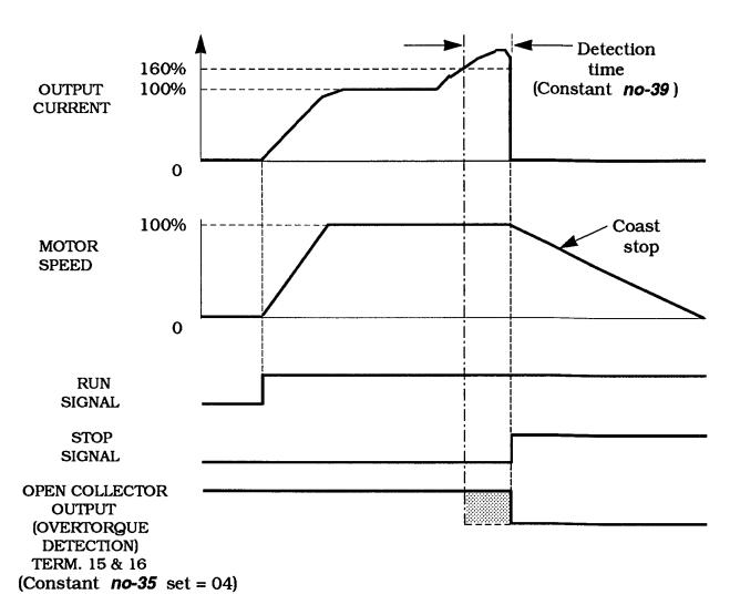
**Overtorque Detection Timing Diagram**
