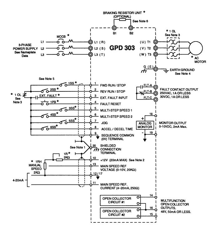
Figure 1-3. Standard Connections (2-Wire Control) (Constant no-00 set to 08)
