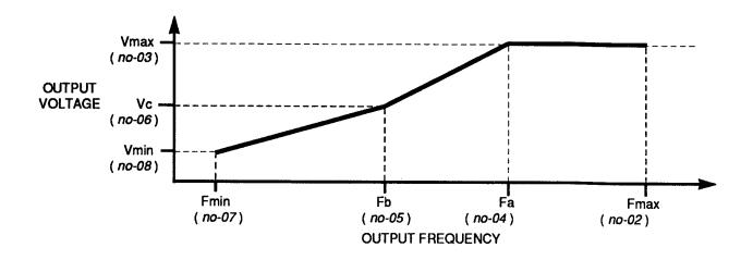
To establish a V/f pattern with a straight line from Fmin to Fa, set Fb = Fmin, and Vc = Vmin.
