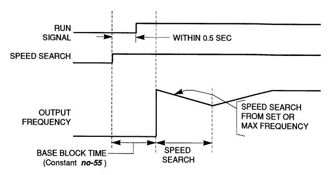
NOTE: When continuous operation mode at momentary stop function is selected, the Speed Search command must be enabled.
