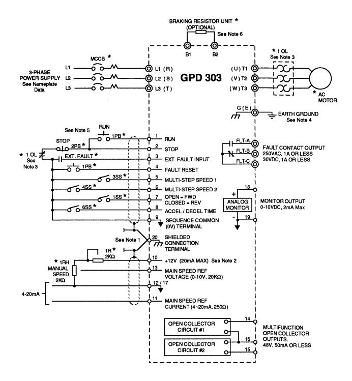
Figure 1-4. Standard Connections (3-Wire Control) (Constant no-00 set to 09)
