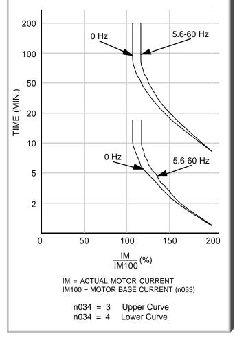
Electronic Motor Thermal Protection Characteristics For General-Purpose Motor
