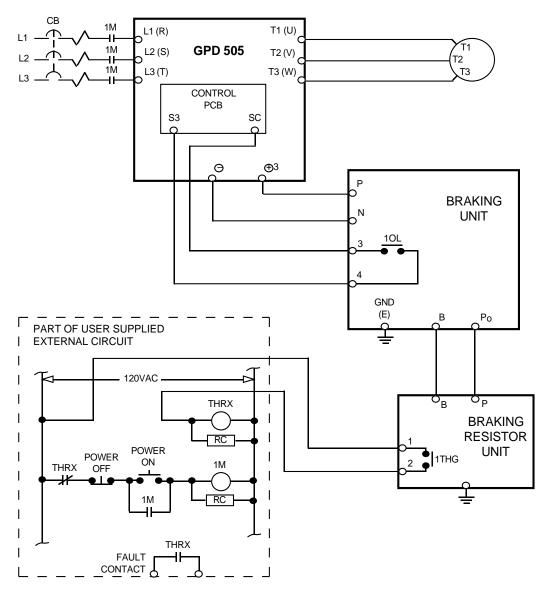
Figure A7-4. Wiring Single Braking Unit and Braking Resistor Unit to Drive
