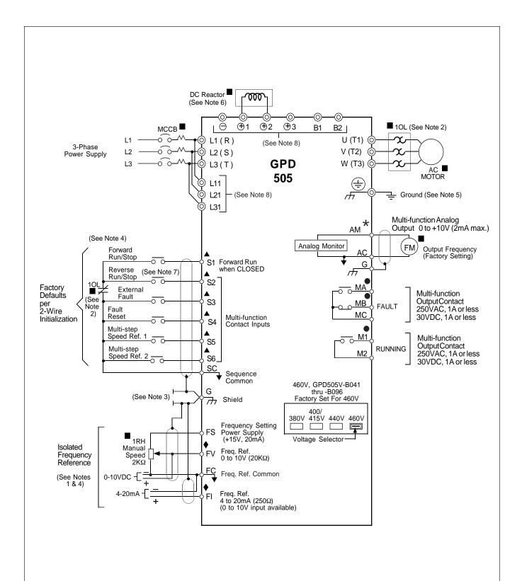
Figure 1-3. 230V or 460V Interconnections - 2-Wire Control (n001 = 8) (with parameters n035 = 0, n036 = 2, n037 = 4, n038 = 9, and n039 = 10)
