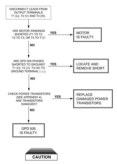
Do not replace DC Bus fuse without first checking output transistors.
