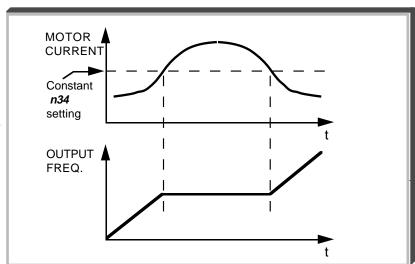
Stall prevention level during accel (constant horsepower) = Stall prevention level during accel  $x \frac{\text{Max. voltage frequency}}{\text{Actual output frequency}}$
