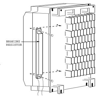
Figure A7-1. Mounting Braking Resistor on Heat Slnk
