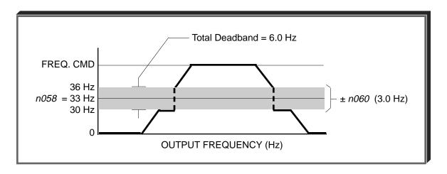
Note that if  $n058 \le n059$  is not satisfied, the Digital Operator displays the parameter setting error code " OPE6 ".
