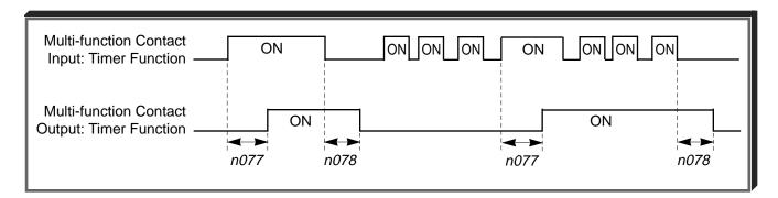
As can be seen, the timer function must be programmed as both a multi-function input **and** an output to be effective.
