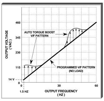
Example of Torque Compensation Operation
