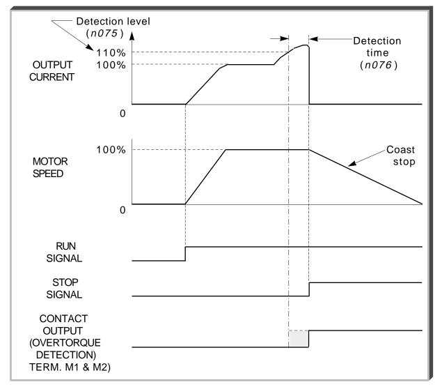
Overtorque Detection Timing Diagram
