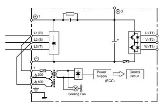
When using DC input as main circuit power, connect control power transformer terminals (r, s400) to L1 and L2, respectively.
