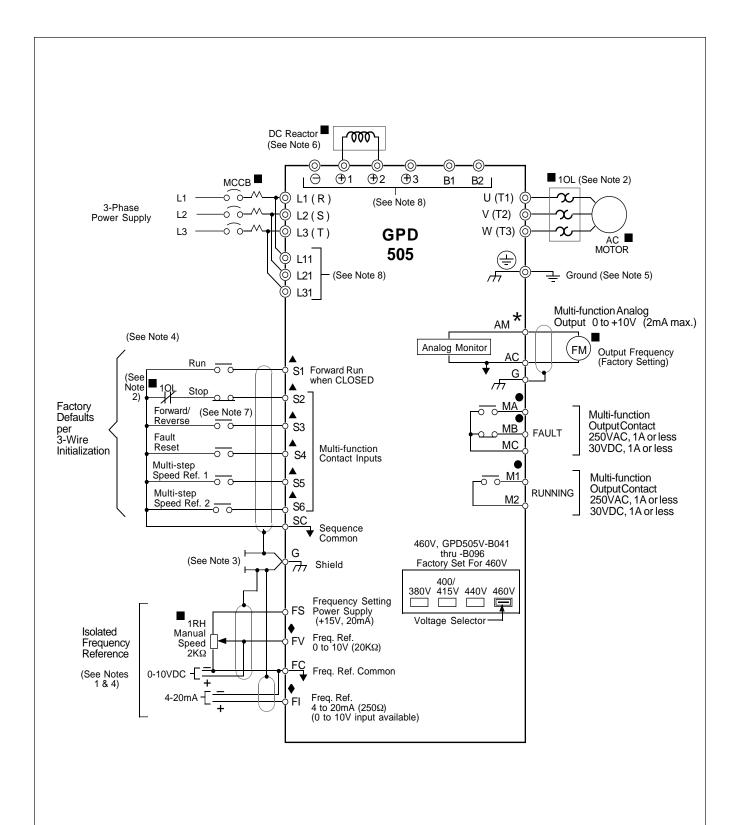
Figure 1-4. 230V or 460V Interconnections - 3-Wire Control (n001 = 9) (with parameters n035 = 1, n036 = --, n037 = 2, n038 = 4, and n039 = 9)
