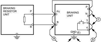
Figure A7-6. Megger Testing Set-up
