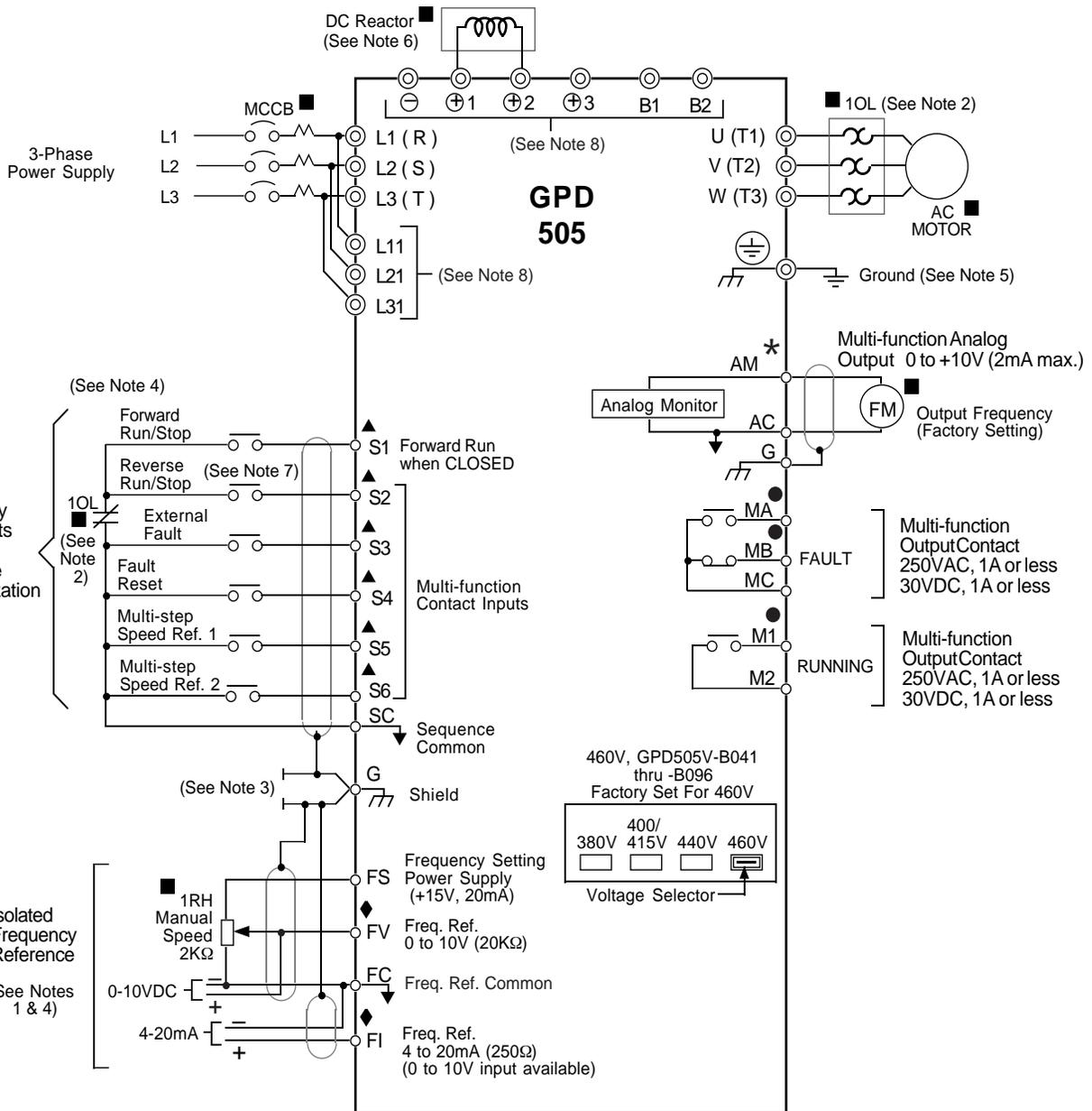
**Figure 1-3. 230V or 460V Interconnections - 2-Wire Control (n001 = 8)
