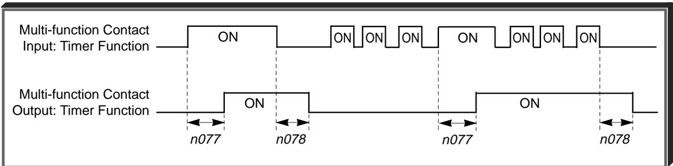
As can be seen, the timer function must be programmed as both a multi-function input **and** an output to be effective.
