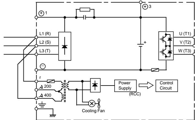
When using DC input as main circuit power, connect control power transformer terminals (r, s400) to L1 and L2, respectively.
