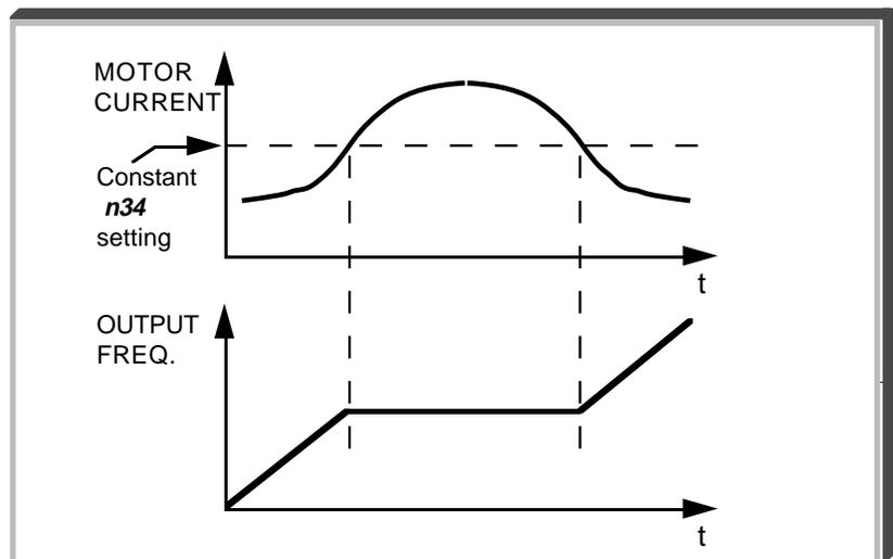
$$\text{Stall prevention level during accel (constant horsepower)} = \text{Stall prevention level during accel} \times \frac{\text{Max. voltage frequency}}{\text{Actual output frequency}}$$
