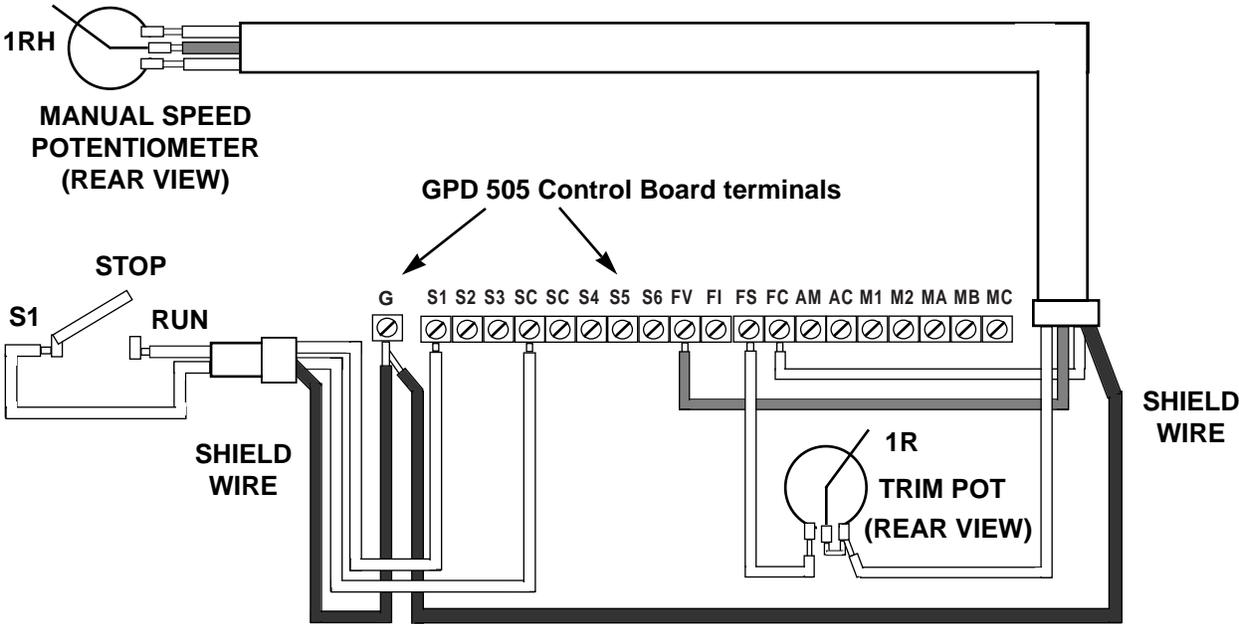
3. Connect a manual speed potentiometer rated 2000-3000 ohms, 1 watt minimum, using three conductor shielded wire, with shield connected at terminal G. Connect wires to the potentiometer as shown, viewing potentiometer from the back. Trace wire shown closest to the top in diagram (right side of potentiometer) and connect to terminal FC. Trace center wire of potentiometer through and connect to terminal FV. The remaining wire will be connected to the trim pot in step 4.
