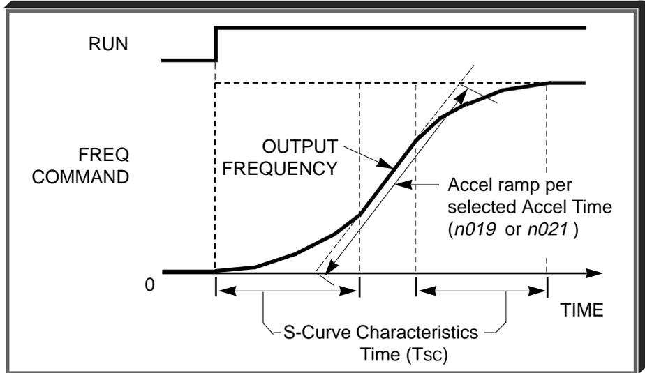
The following figure shows FWD/REV switching and acceleration & deceleration to a stop with S-curve active.
