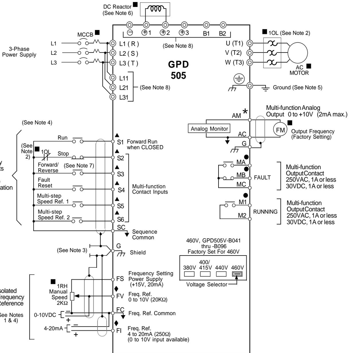
**Figure 1-4. 230V or 460V Interconnections - 3-Wire Control (n001 = 9)
