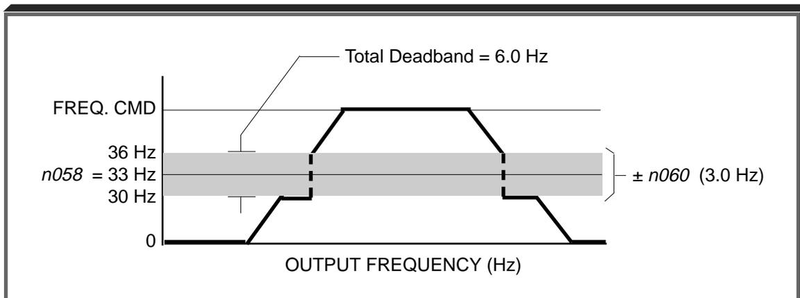
Note that if  $n058 \leq n059$  is not satisfied, the Digital Operator displays the parameter setting error code " **OPE6** ".
