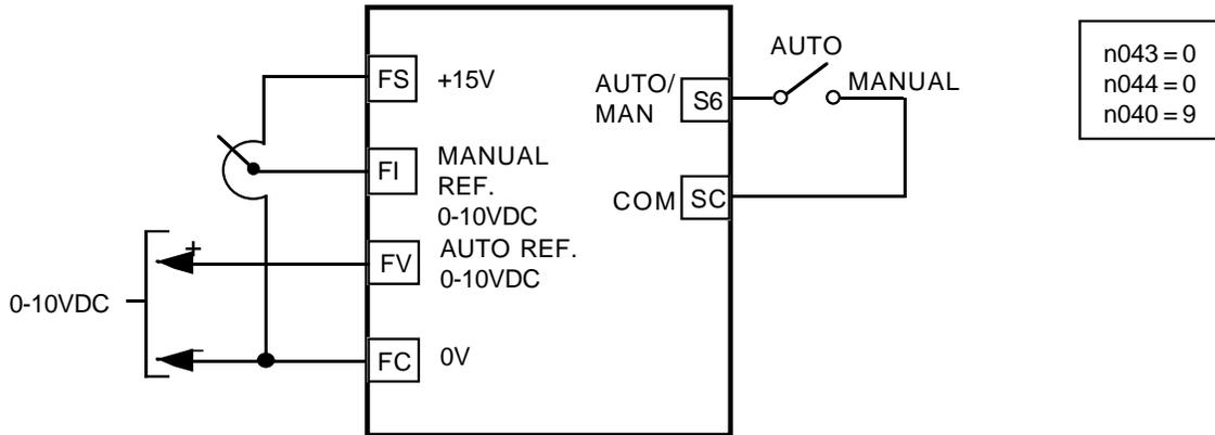
D. 4-20mA DC signal (auto) and 0-10VDC signal or speed pot (manual):
