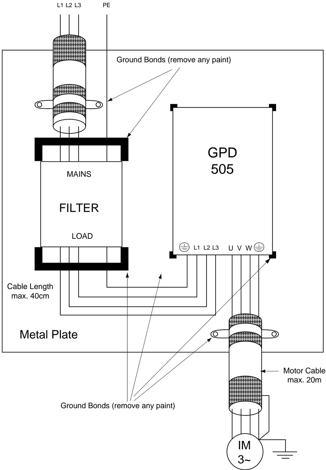
**Figure 1-2A. Installation of Line Filter and GPD 505 Drive**
