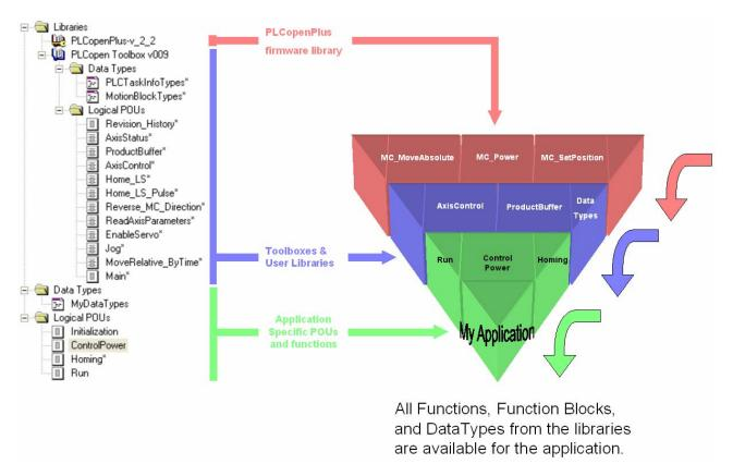
Function, Function Blocks, and Data Types provided in the fimware and user libraries speed code development for the application programmer. At the application level, the programmer can pull from the resources provided in the included libraries.
