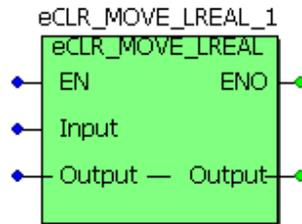
Figure 33: LREAL move with enable logic
