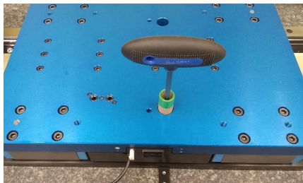
Figure 3. Screw Insertion Tube Example
