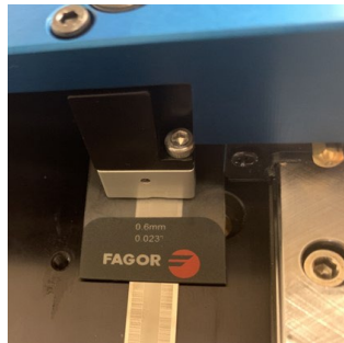
Figure 3: Shim placement between readhead and scale
