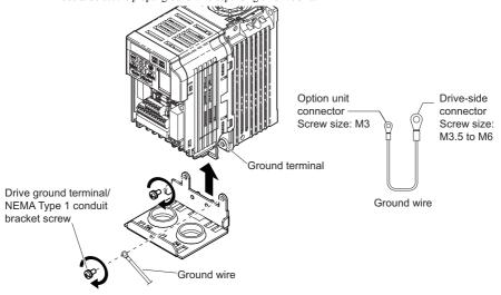
Figure 11 Reattach the NEMA Type 1 Conduit Bracket and Connect the Ground Wire
