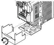
Figure 8 Remove the NEMA Type 1 Terminal Cover
