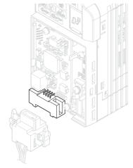
Figure 3 Communication Cable Connector
