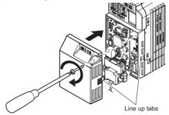
Figure 19 Attach the Option Cover
