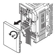
Figure 4 Remove the Front Cover
