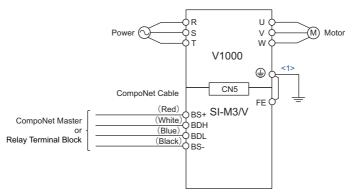
Figure 18 Wiring Diagram
