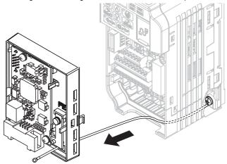
Figure 15 Ground Wire Routing
