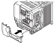
Figure 13 Reattach the Terminal Cover (Models CIMR-V□BA0006□ to BA0018□; 2A0008□ to 2A0069□; 4A0001□ to 4A0038□)
