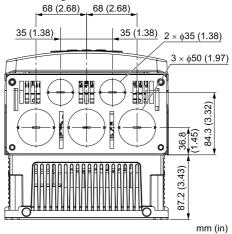
Figure 5.16 Knock-Out Hole Dimension Diagram 4
