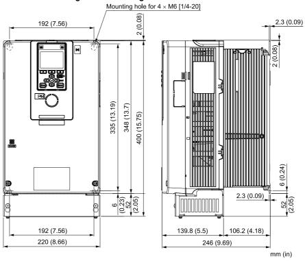
Figure 5.6 Dimension Diagram 6
