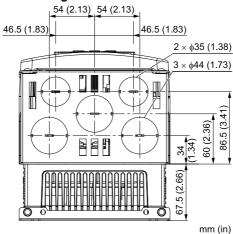
Figure 5.15 Knock-Out Hole Dimension Diagram 3
