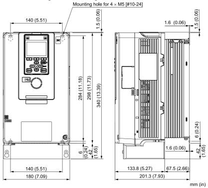
Figure 5.3 Dimension Diagram 3
