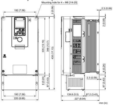
Figure 5.5 Dimension Diagram 5
