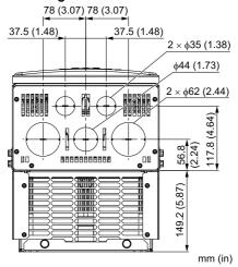
Figure 5.21 Knock-Out Hole Dimension Diagram 9
