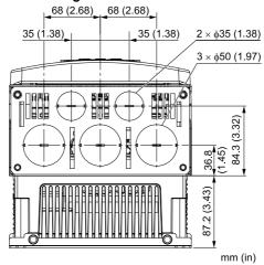
Figure 5.17 Knock-Out Hole Dimension Diagram 5
