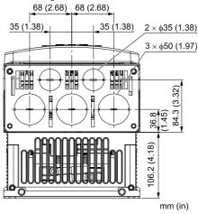
Figure 5.18 Knock-Out Hole Dimension Diagram 6
