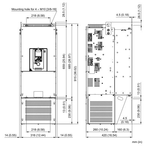
Figure 5.11 Dimension Diagram 11
