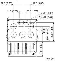
Figure 5.23 Knock-Out Hole Dimension Diagram 11
