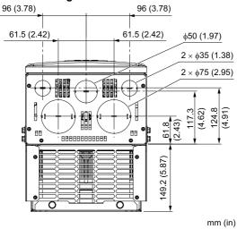
Figure 5.22 Knock-Out Hole Dimension Diagram 10
