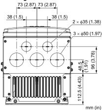
Figure 5.19 Knock-Out Hole Dimension Diagram 7
