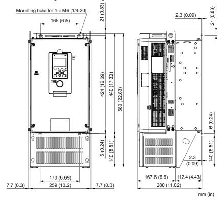
Figure 5.8 Dimension Diagram 8
