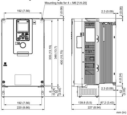
Figure 5.4 Dimension Diagram 4
