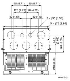
Figure 5.24 Knock-Out Hole Dimension Diagram 12
