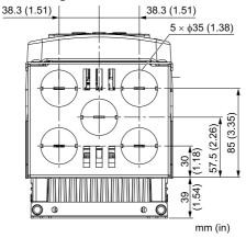
Figure 5.13 Knock-Out Hole Dimension Diagram 1
