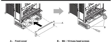
Figure 5.33 Install the Front Cover
