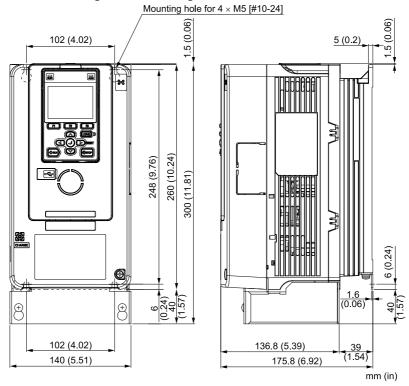
Figure 5.1 Dimension Diagram 1
