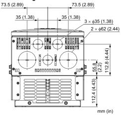
Figure 5.20 Knock-Out Hole Dimension Diagram 8
