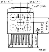
Figure 5.14 Knock-Out Hole Dimension Diagram 2
