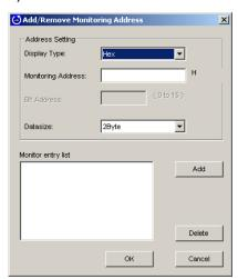
4) Enter the necessary items and click "Add". If the addresses entered can be accessed, then those items will be added to the list of monitors. If access is not possible, a message will appear that indicates that the address entered is not allowed. Click "OK" to return to the "Add/Delete Monitor Address" window.
