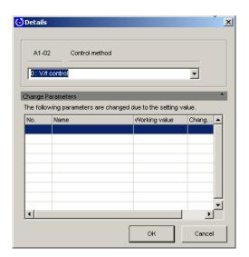
Either select the setting value from the List Box, or enter the value directly. Any parameters that are affected when the control mode is changed will be displayed in this list.
