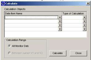
3) Use the drop-down menu to select the parameter in the Data column, and then the type of calculations on the right.
