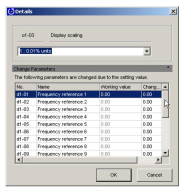
Either select the desired setting from the drop-down menu or enter the setting manually.
