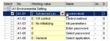
The value will be displayed, provided the value is within the possible setting range, and all parameters with that access level will appear in the parameter list.
