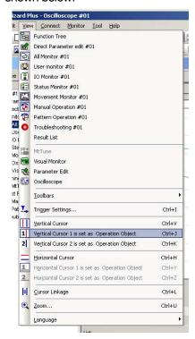
3) After selecting, "Vertical Cursor 1 is set as Operation Object", click on the graph to position the cursor.
