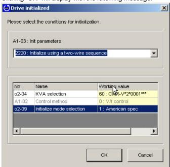
Either select the type of initialization from the drop-down menu or enter the value manually. Next, either select "Current Setting Value" from the drop-down menu that appears below, or enter the value manually.
