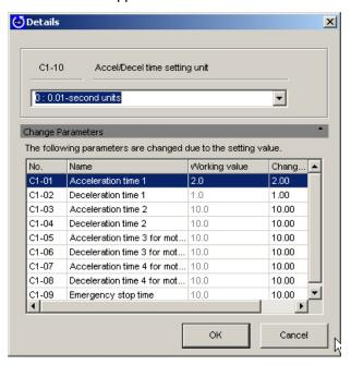
Either select the setting value from the List Box, or enter the value directly. Any parameters that are affected when the change is made will be displayed in this list.
