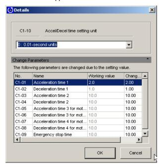
Either select the setting value from the List Box, or enter the value directly. Any parameters that are affected when the change is made will be displayed in this list.
