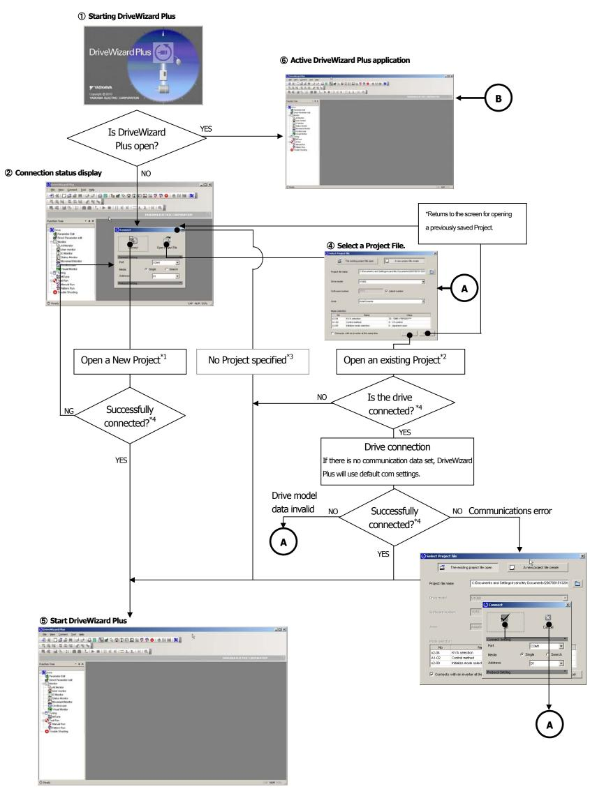
\*1 New Project: DriveWizard Plus creates a new Project file and automatically assigns default values to all parameters.
