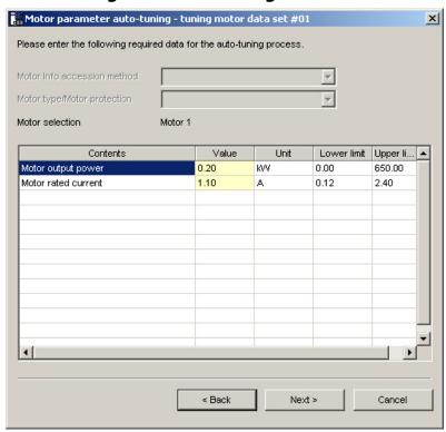
The information required can be obtained from the motor nameplate or from the motor test report. Enter the data required into the appropriate column.
