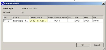
• Display the Parameter Edit window from the Analog Input Parameter.
