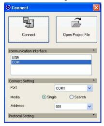
If DriveWizard Plus is unable to communicate with the drive, the window above will not appear and the following message will be displayed instead:
