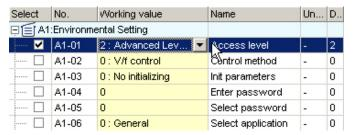
The value will be displayed, provided the value is within the possible setting range and all parameters with that access level will appear in the parameter list.
