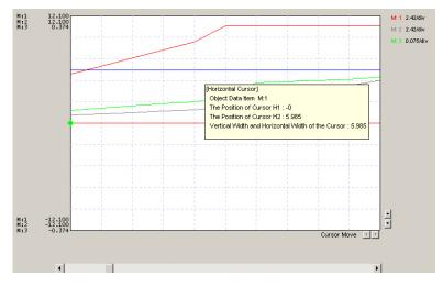
6) Move the cursor by selecting "Cursor Linkage (<u>C</u>)" from the View (V) menu and then adjusting the space between both cursors using the mouse.
