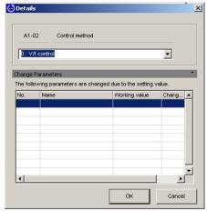
Either select the setting value from the List Box, or enter the value directly. Any parameters that are affected when the control mode is changed will be displayed in this list.
