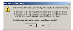
To accept the operation pattern that has been set until the drive reaches zero speed, click "Yes". To return to the Pattern Run window and start over again, click "No".
