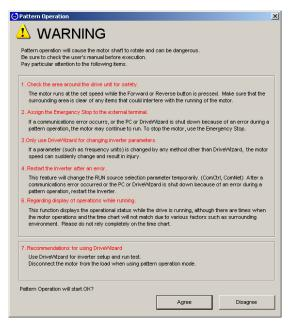
Click "Agree" to begin rotating the motor. Clicking on "Disagree" will stop the operation and the motor will not rotate.
