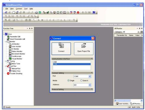
The first window to appear asks if the user would like to connect to a drive or open up a Project file.
