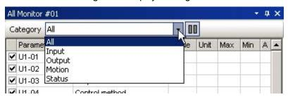
This example shows the Monitor display after selecting to view Input monitors.
