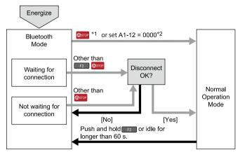
Figure 5.5 Changing between Bluetooth Mode and Normal Operation Mode
