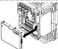
Figure 5.24 Remove the Front Cover
