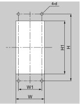
Figure 5.38 Internal/Flush-Mount Enclosure Panel Cut-Out Dimensions
