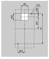
Figure 5.34 External/Face Mount Enclosure Panel Cut-Out
