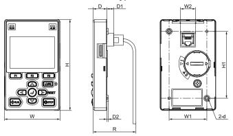
Figure 5.9 Exterior and Mounting Dimensions
