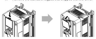
Figure 5.1 Remove the Keypad
