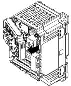
Figure 5.32 Removing the Included Drive Keypad
