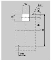
Figure 5.10 External/Face Mount Enclosure Panel Cut-Out Dimensions
