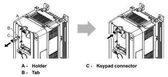
Figure 5.13 Moving the Keypad Connector to the Holder
