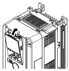
Figure 5.2 Attach the Keypad
