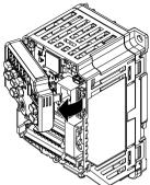
Figure 5.25 Removing the Included Drive Keypad
