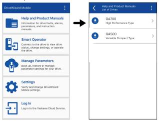
Before you go to the next step, make sure that you get the Bluetooth ID from parameter A1-12 in the drive that you will connect to DriveWizard Mobile. You must enter the Bluetooth ID into DriveWizard Mobile in Step 8.
