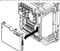
Figure 5.31 Remove the Front Cover
