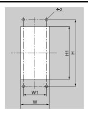
Figure 5.27 Internal/Flush-Mount Enclosure Panel Cut-Out Dimensions
