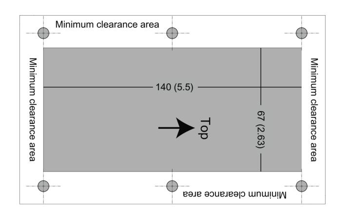
Measure the printed dimensions before you drill the screw holes Moisture can cause the template scale to change  $\triangleright$
