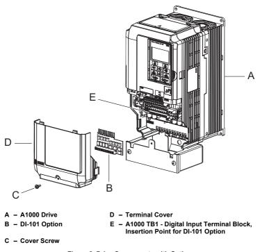
Figure 2 Drive Components with Option
