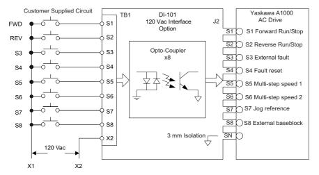
Figure 8 Wiring Diagram Example
