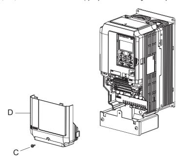
Figure 3 Terminal Cover Removal
