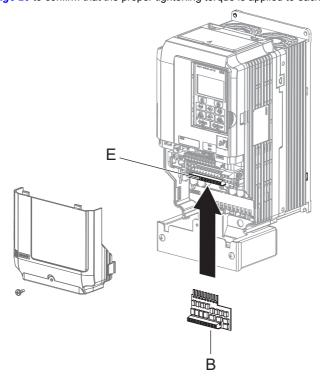
Figure 5 DI-101 Option Insertion into TB1
