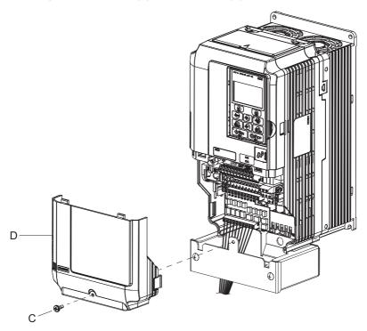
Figure 9 Replace the Terminal Cover
