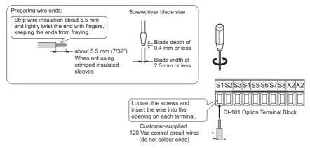
Figure 7 Preparing Cable Wiring
