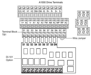
Figure 6 DI-101 Option to Drive Connection
