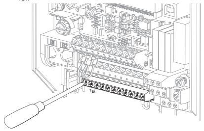
Figure 4 Loosen Drive Control Terminals TB1 S1 to S8 and SN
