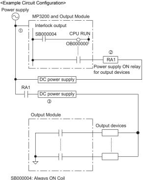
(ON while the CPU Unit is operating normally.) OB000000: Interlock output
