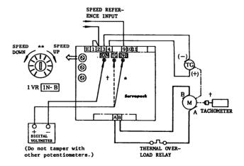
Fig. 13 Changing of Rated Reference Voltage
