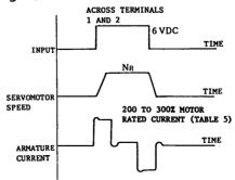
Fig. 8 Servomotor Start-Stop Characteristics
