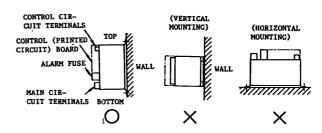
Fig. 3 Mounting Direction of Servopack
