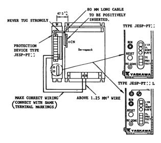
Fig. 17 Mounting and Connection of Servopack and Protection Device
