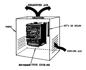
Fig. 1 Typical Layout for Panel Mounting
