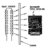
Fig. 2 Protection against Heat Radiation
