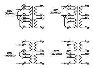
Fig. 5 Connection of Power Transformer
