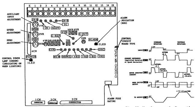
Fig. 10 Arrangement of Potentiometers and Check Terminals
