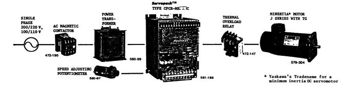
Table 1 Combination of Servopack and Servomotors and Optional Components
