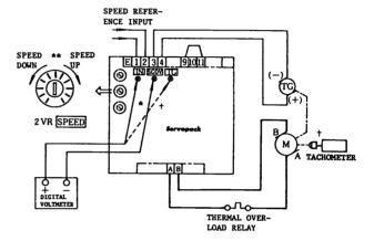
Fig. 12 Setting of Motor Speed
