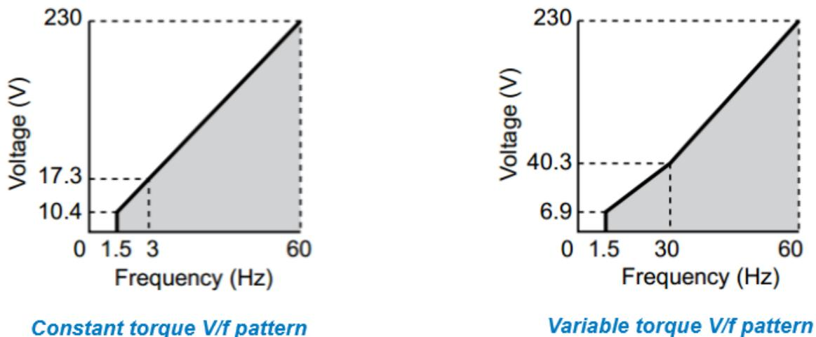
Figure 2: Figure 2: Different V/f patterns allow a VFD to control a multitude of different applications while maintaining optimal performance
