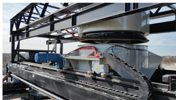
**The system distributes asphalt to the 6 truck load-out silos.**
