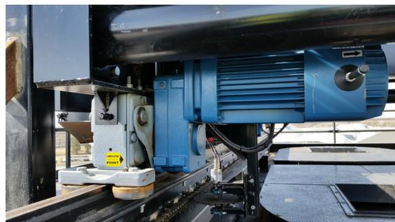
**The traveling batcher drive is designed for unloading the batch into each load.**
