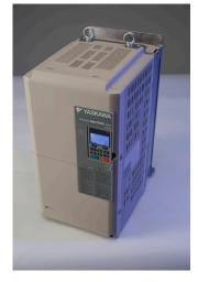
The Yaskawa U1000's unique AC-to-AC power conversion architecture is the latest advancement in IEEE 519 low-harmonic variable frequency drives. By eliminating the DC bus the U1000 is smaller and more efficient than earlier products.
