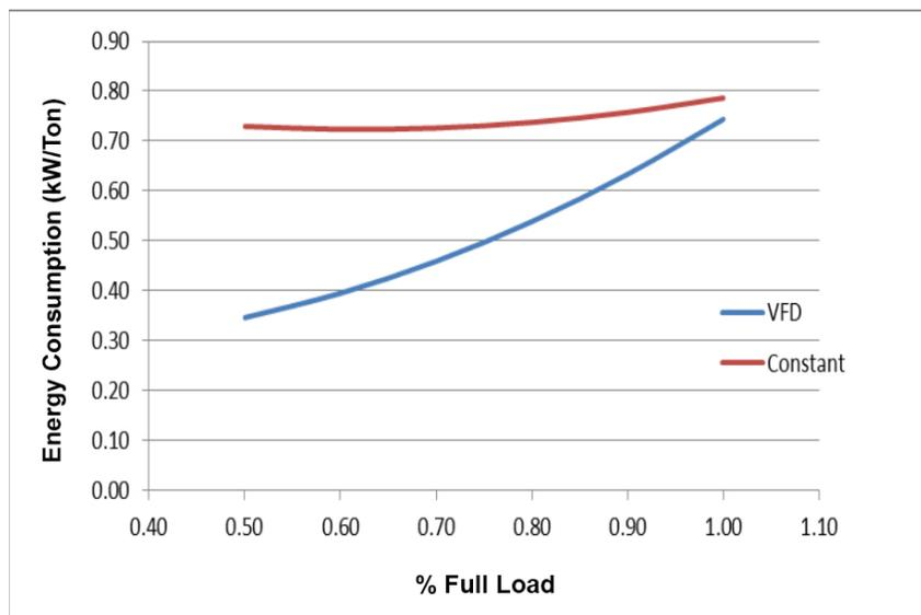
Figure 2: General system differences in efficiency between a constant speed chiller compared with that of a VFD operated chiller.
