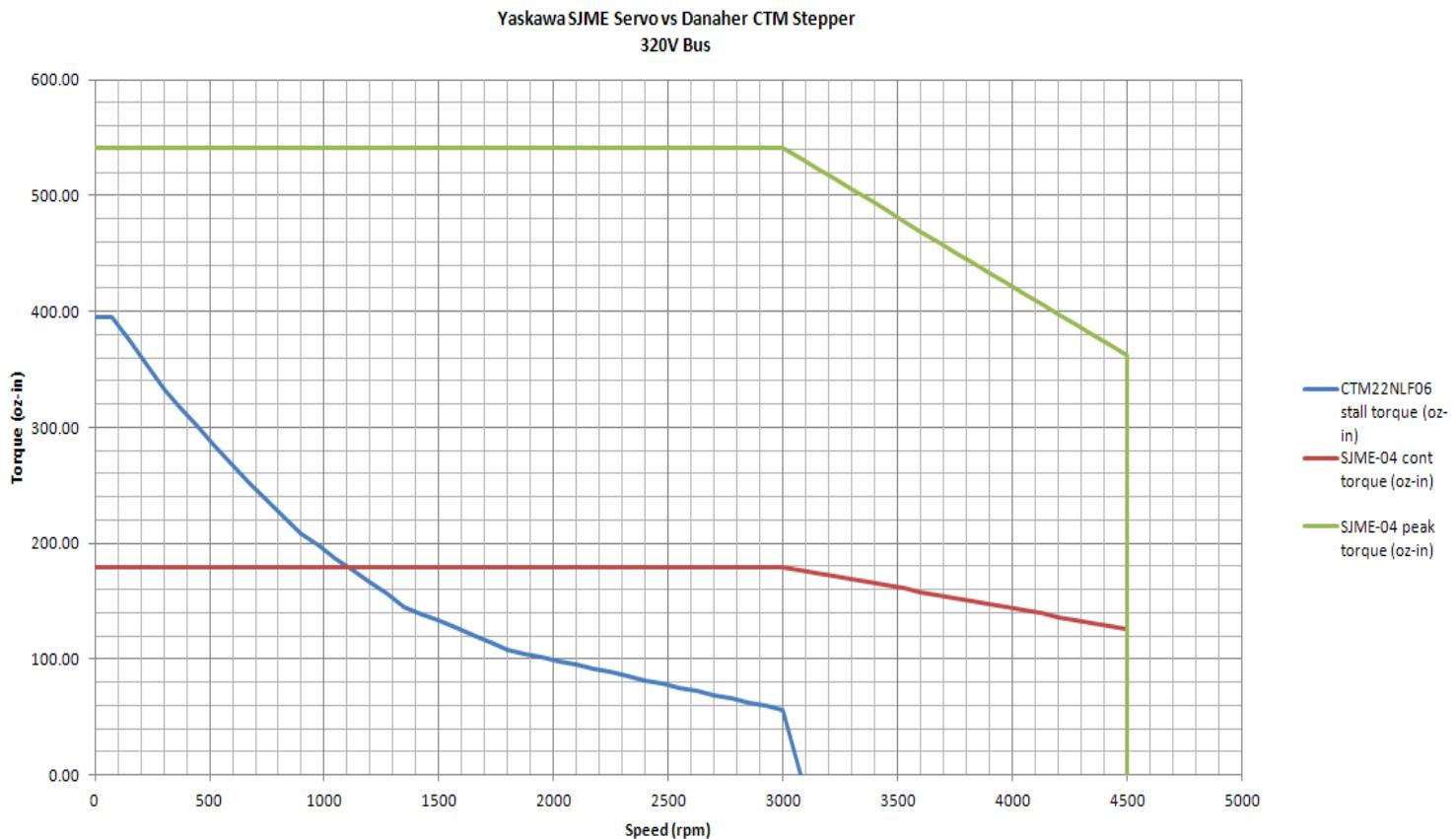
Another inherent disadvantage of stepper motors is the existence of two distinct instability regions. There is a low speed region of instability, typically between 100 and 300 full steps per second or 30 to 90 rpm, that results from the excitation of the natural frequency of the motor. When the motor is operated in this region, there will be a large velocity ripple and a potential loss of steps and position.
