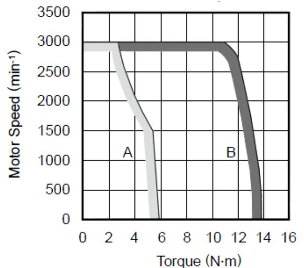
Figure 1 - Typical Torque-Speed Curve with continuous (A) & intermittent (B) duty zones shown
