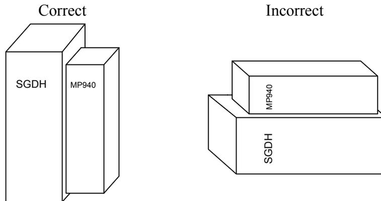
***Figure 2.1: Mounting Orientation***
