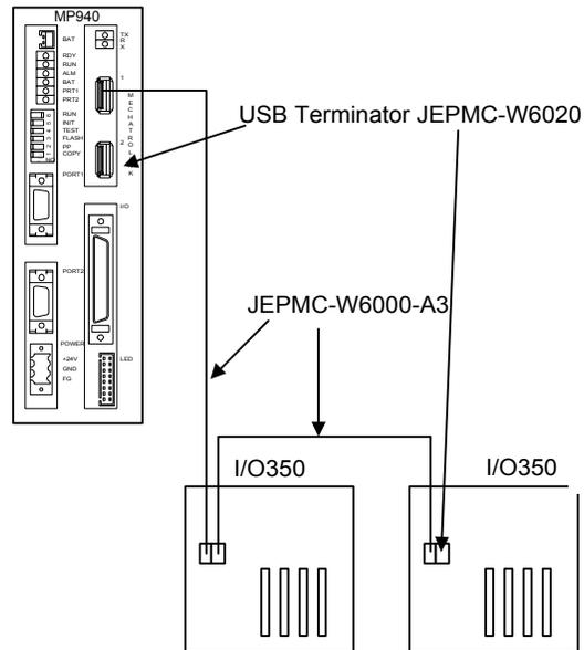
**Figure 5.7: MP940 Connection to Multiple I/O 350 Modules**
