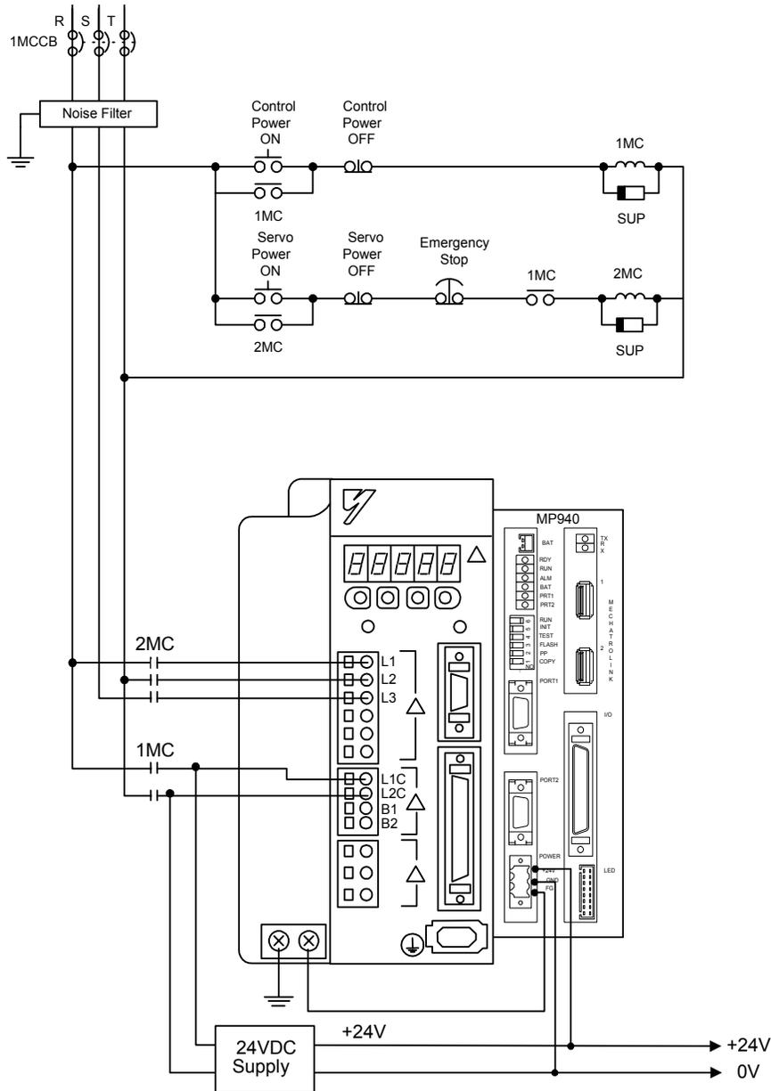
Figure 2.9: Three-phase Wiring
