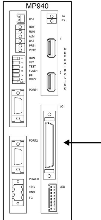
*Figure 6.1: Digital I/O Connection*
