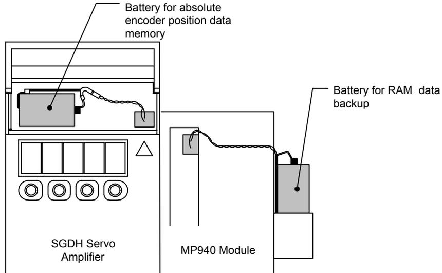
**Figure 2.6: MP940 and SGDH Batteries**
