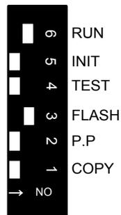
*Figure 3.3: Transfer from Flash Memory to RAM*
