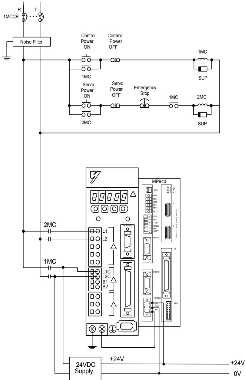
Figure 2.8: Single-phase Wiring
