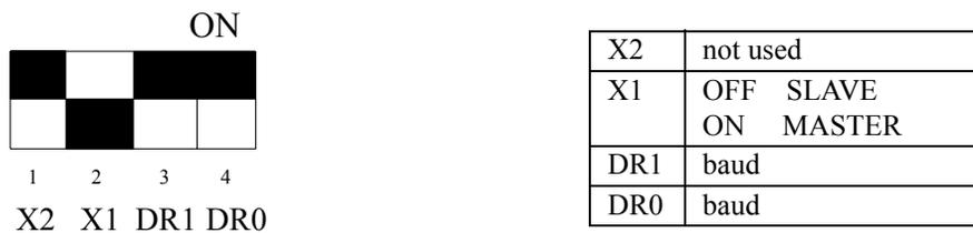
**Figure 5.10: DIP Switches**
