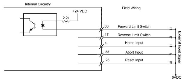
X axis dedicated inputs shown. Other axes are the same. Check CN5 connector for pin configuration.
