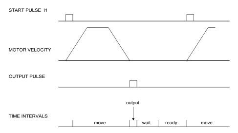
Motor Velocity and the Associated Input/Output Signals
