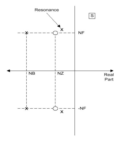
Resonance shows up as a pair of complex poles with a real part. A notch filter attempts to cancel the unwanted poles by placing zeroes on top of them and placing new poles in a more desirable location. The following diagram shows the pole-zero configuration of a general system with resonance and a notch filter:
