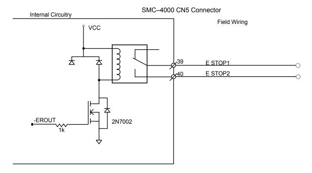
The SMC-4000 closes the relay contact under normal operating conditions. The relay is controlled by the same circuit as the error LED. The relay will be open if the error LED is ON.
