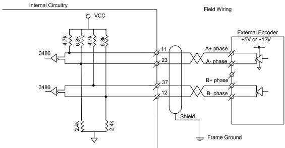
X axis internal encoder shown See 5CN connector for other axis pin connections.
