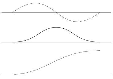
Velocity Profile with Sinusoidal Acceleration
