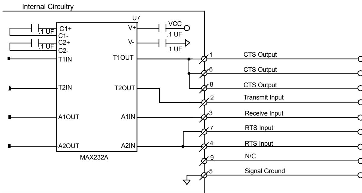
**NOTE:** Hardware handshaking must be used with the SMC-4000. If it is impossible to implement hardware handshaking, use a jumper between pins 1 and 4 in the connector.
