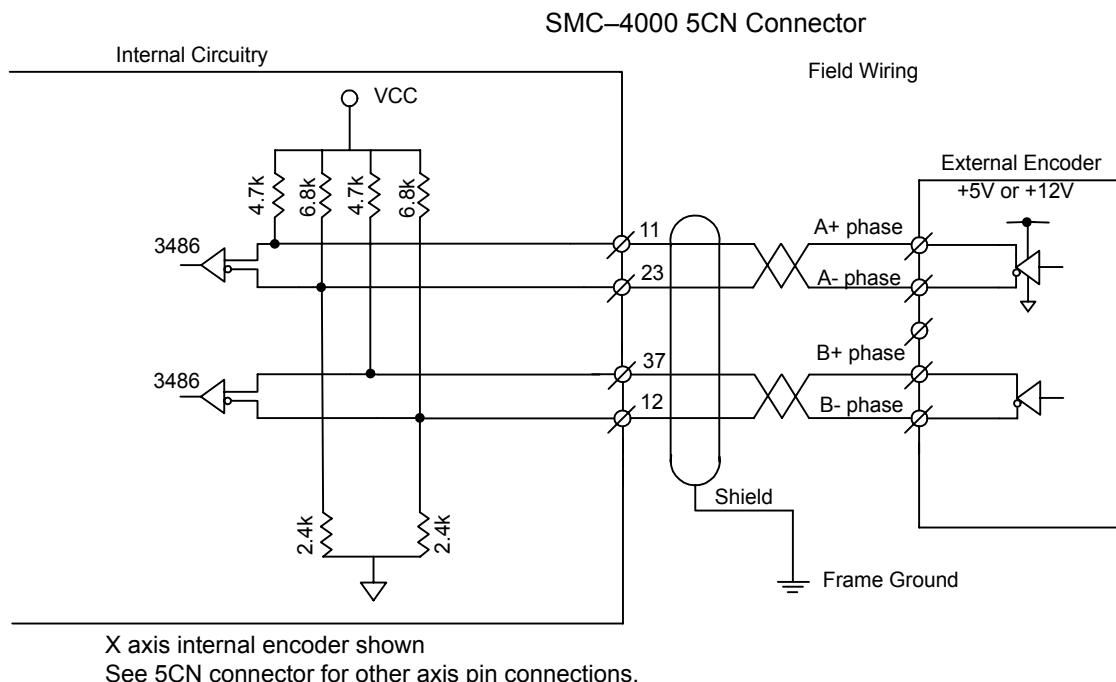
Standard voltage levels are TTL (0V to 5V), however, voltage levels up to 12V are acceptable. If using differential 12V signals, no modification is required. Single ended 12V signals require a bias voltage applied to the complimentary input, i.e.; use two 10k resistors, one connected to +12V and the other connected to the encoder signal ground to hold the /A phase and /B phase at 6VDC. Do not use a 24VDC encoder.
