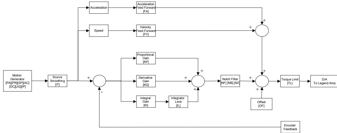
The elements of a servo system include the motor, driver, encoder and the controller. These elements are shown in the following illustration. The mathematical model of the various components is given below:
