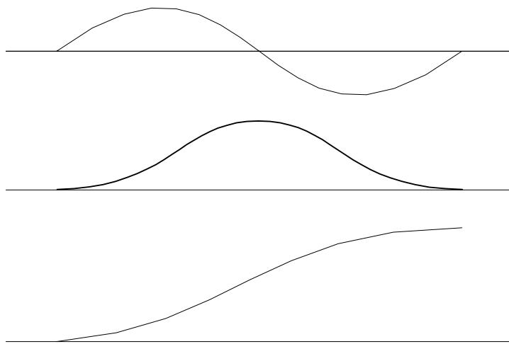
***Velocity Profile with Sinusoidal Acceleration***
