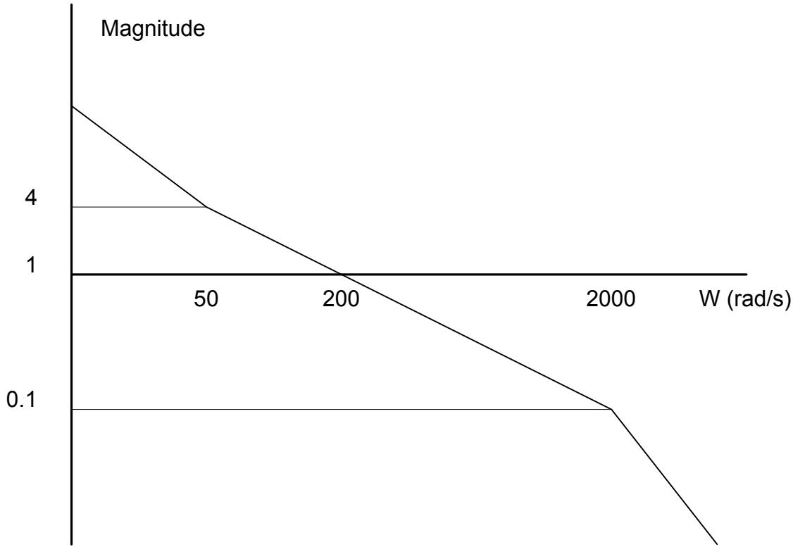
*Bode plot of the open loop transfer function*
