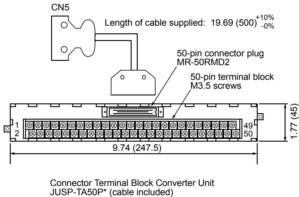
Connector Terminal Block Converter Unit
