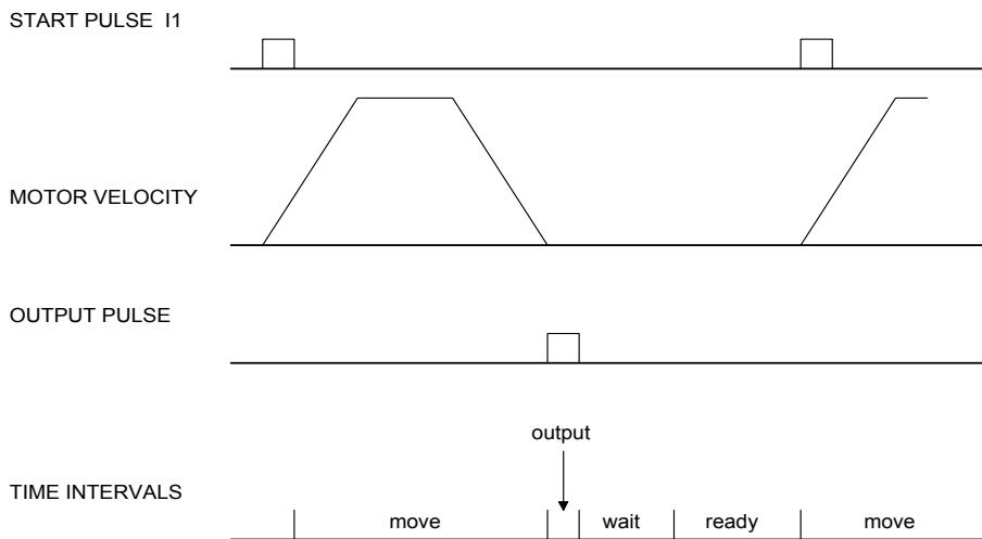
***[Motor Velocity and the Associated Input/Output Signals](#)***
