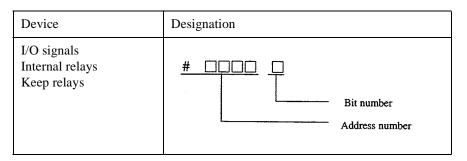
In this case, the address number has the same meaning as a) explained above, and it can be considered to be the name assigned collectively to eight points of a signal.
