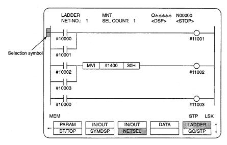
Fig. 8.2 Ladder Diagram Display Screen
