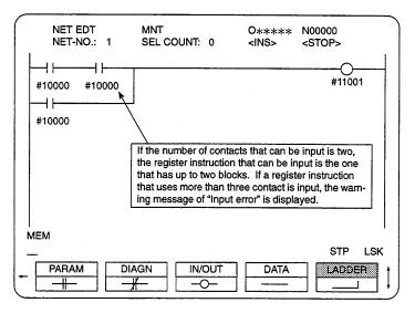
Fig. 8.16 Input Position of Register Instruction
