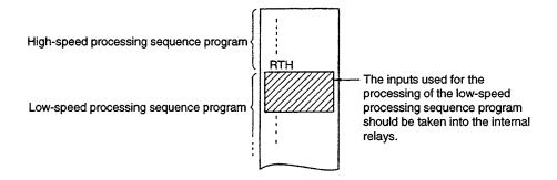
Fig. 4.4 Low-speed Processing Sequence Program
