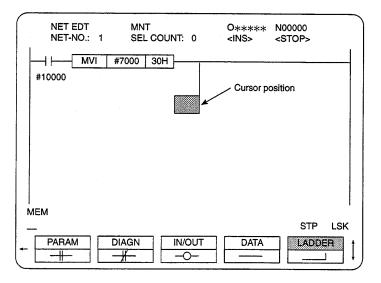
Fig. 8.12 Drawing a Vertical Line
