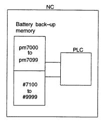
Fig. 5.1 Handling of PCNC Sequence Program
