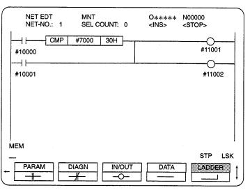
Fig. 8.18 Incorrect Net (More than One Ladder)
